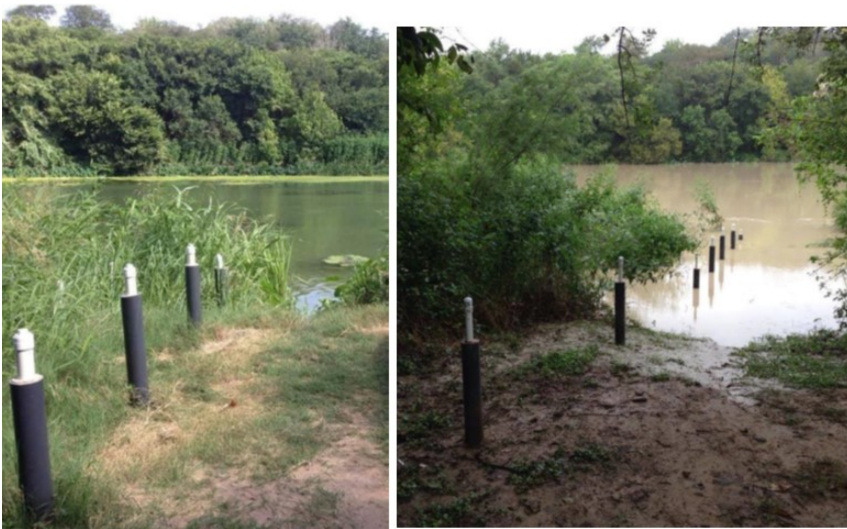
Figure 7-2. Network of monitoring wells installed in the Colorado River alluvium at Hornsby Bend using a Geoprobe System under flow conditions (A) and after a 10,000-cubic-feet-per-second storm event (B) (from Barrera, 2015).
