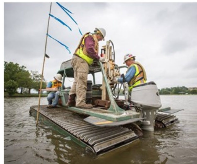
Figure 7-10. Examples of Geoprobe Rigs (provided courtesy of Vortex Drilling, Inc in San Antonio, Texas and Pro-Tech in Baton Rouge, Louisiana).
