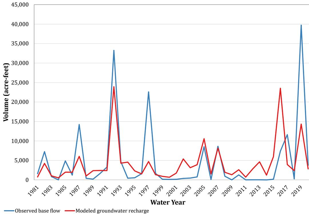
**Figure 7-7. Comparison of recharge simulation results to observed base flow for gauge 08086212 (Middle Brazos-Millers).**
