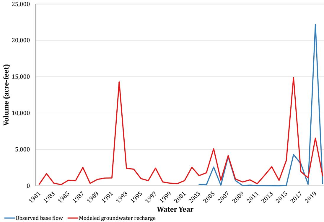
**Figure 7-7. Comparison of recharge simulation results to observed base flow for gauge 08086050 (Middle Brazos-Millers).**
