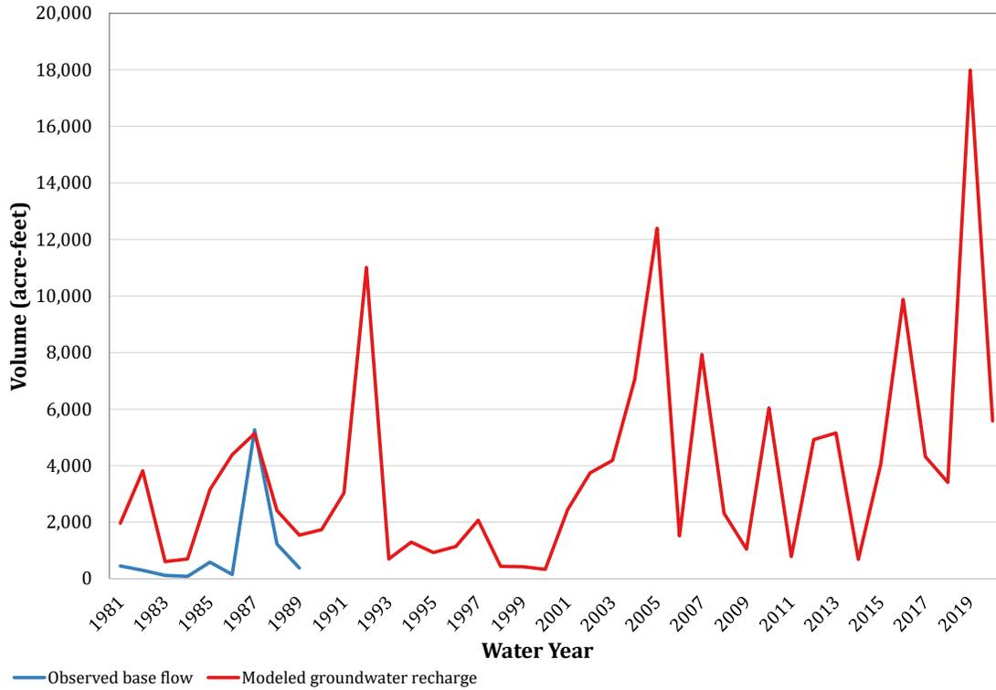
**Figure 7-?. Comparison of recharge simulation results to observed base flow for gauge 08083245 (Upper Clear Fork-Brazos).**
