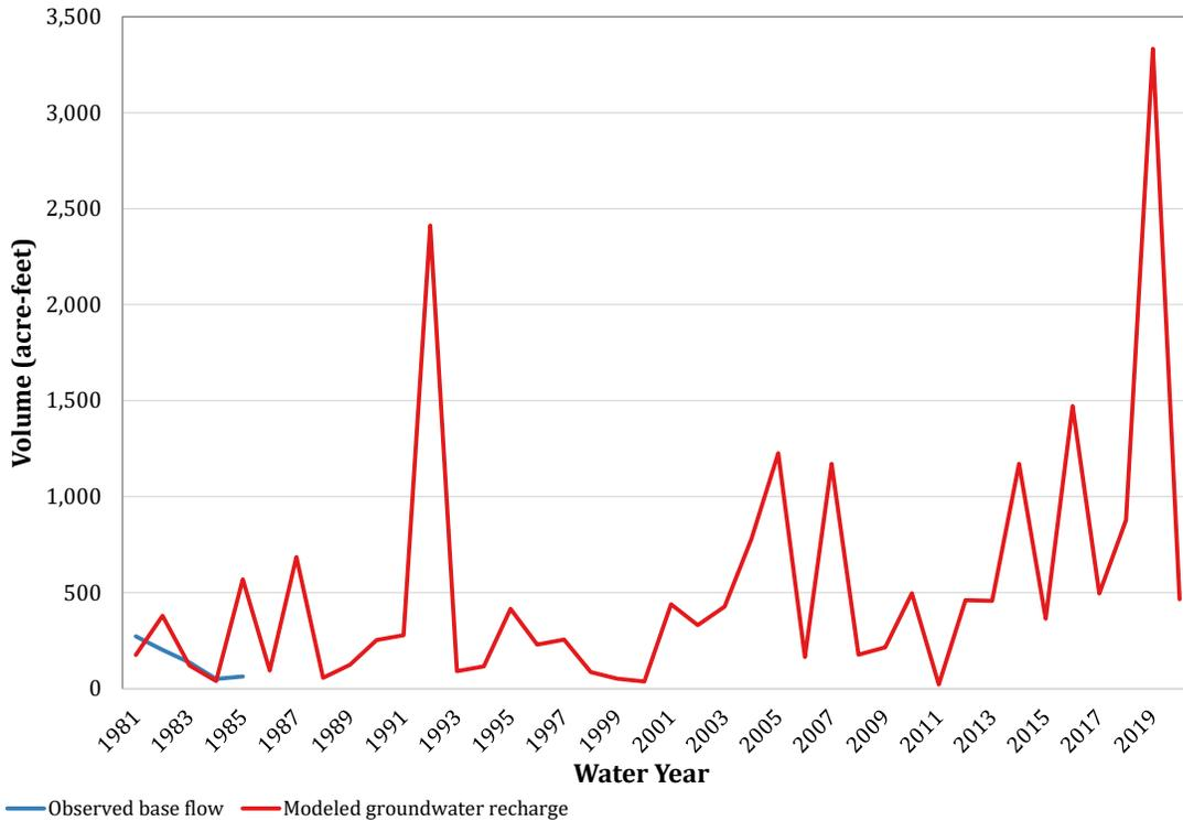
**Figure 7-7. Comparison of recharge simulation results to observed base flow for gauge 08144800 (San Saba).**
