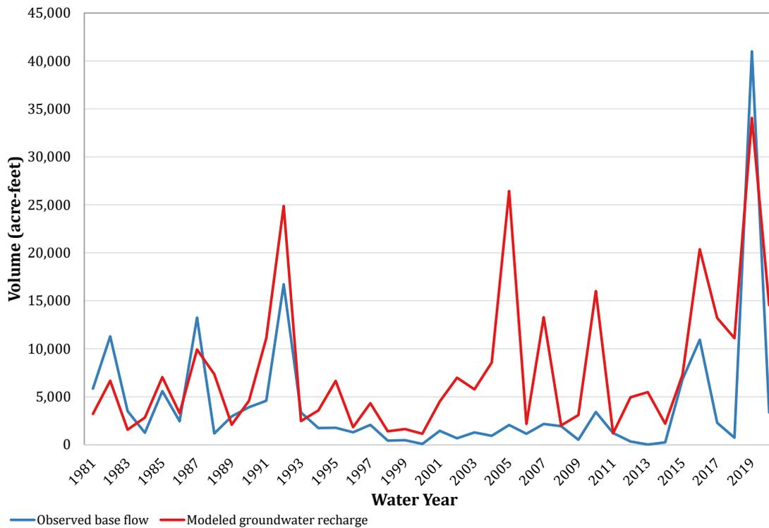
**Figure 7-?. Comparison of recharge simulation results to observed base flow for gauge 08084800 (Upper Clear Fork-Brazos).**
