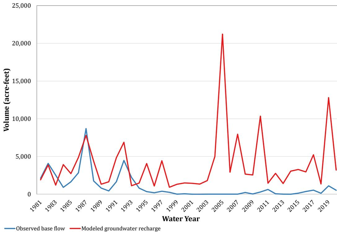
**Figure 7-?. Comparison of recharge simulation results to observed base flow for gauge 08083100 (Upper Clear Fork-Brazos).**
