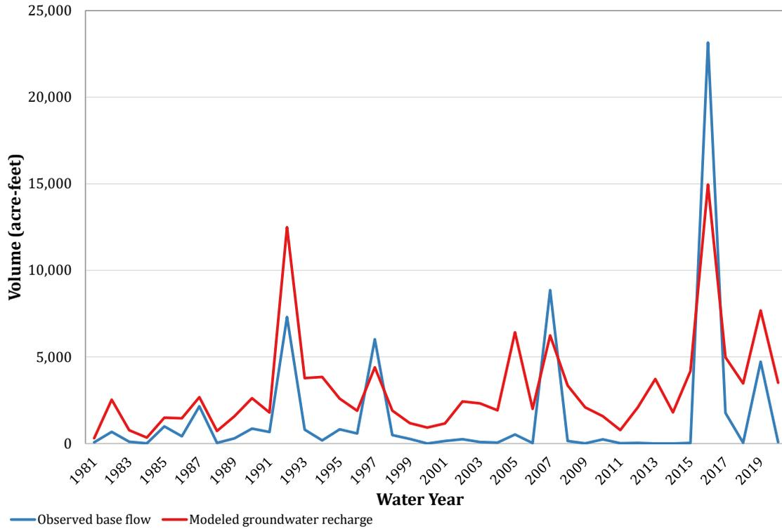
**Figure 7-7. Comparison of recharge simulation results to observed base flow for gauge 08086290 (Middle Brazos-Millers).**
