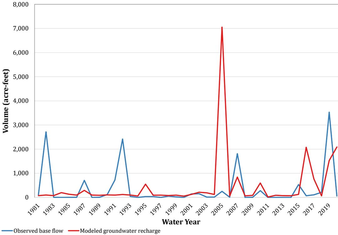
**Figure 7-?. Comparison of recharge simulation results to observed base flow for gauge 08082700 (Middle Brazos-Millers).**
