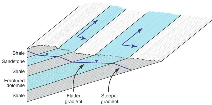
**Figure 12-2. Illustration of regional-scale anisotropy within layered formation of alternating higher and lower hydraulic conductivity. Magnitudes of permeability indicated conceptually by the lengths of the arrows.**
