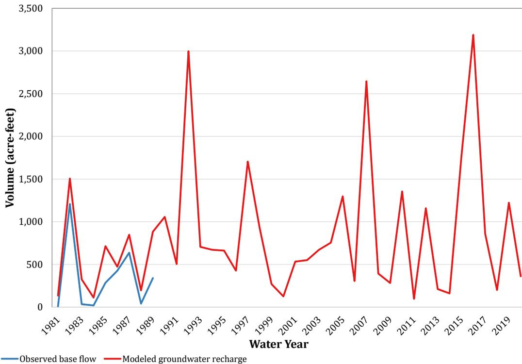
**Figure 7-7. Comparison of recharge simulation results to observed base flow for gauge 08088450 (Middle Brazos-Palo Pinto).**
