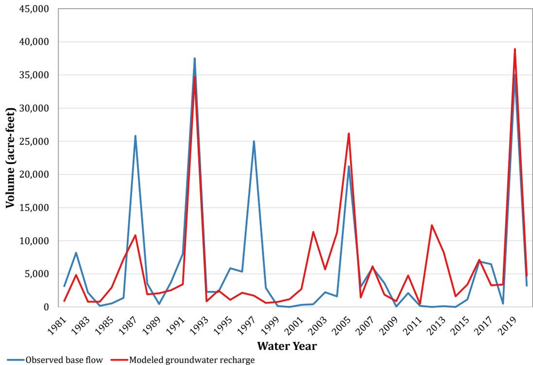
**Figure 7-?. Comparison of recharge simulation results to observed base flow for gauge 08127000 (Middle Colorado).**
