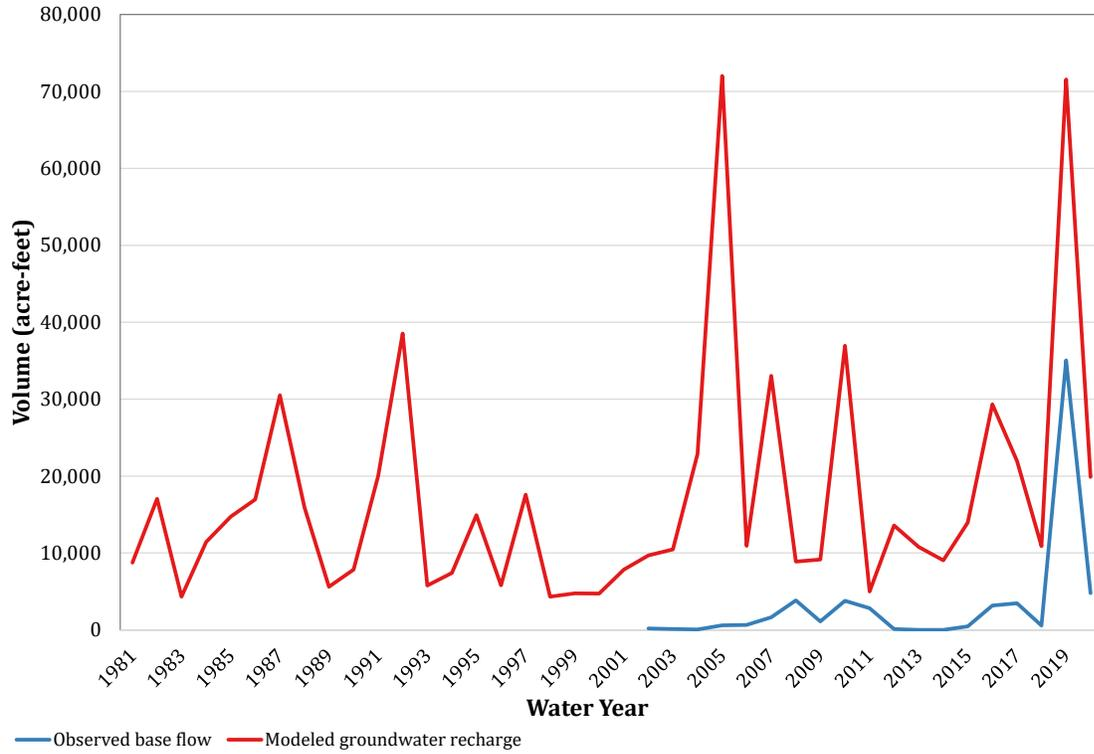
**Figure 7-7. Comparison of recharge simulation results to observed base flow for gauge 08083230 (Upper Clear Fork-Brazos).**
