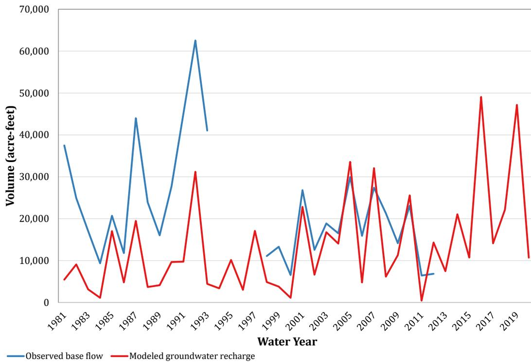
**Figure 7-?. Comparison of recharge simulation results to observed base flow for gauge 08144600 (San Saba).**
