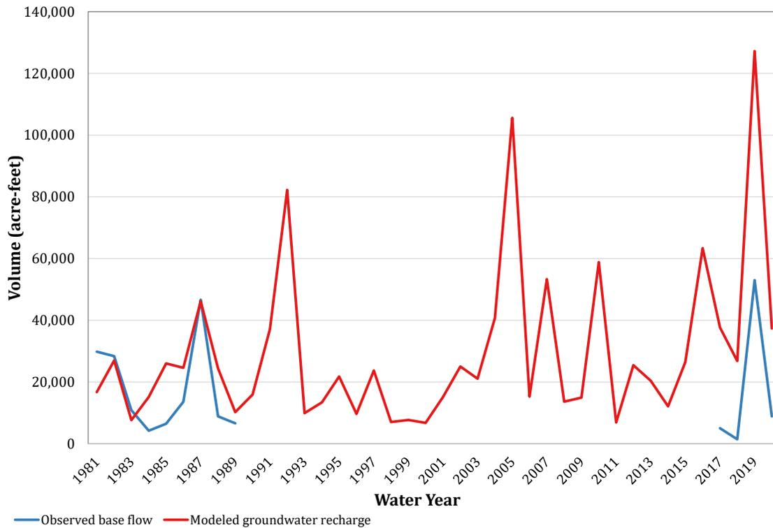
**Figure 7-7. Comparison of recharge simulation results to observed base flow for gauge 08083240 (Upper Clear Fork-Brazos).**
