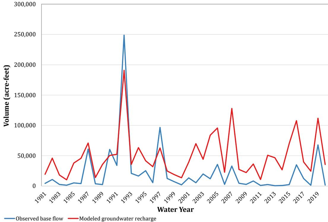
**Figure 7-?. Comparison of recharge simulation results to observed base flow for gauge 08143600 (Middle Colorado).**
