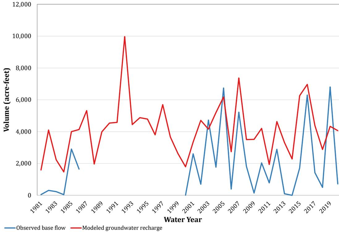
**Figure 7-?. Comparison of recharge simulation results to observed base flow for gauge 08099300 (Middle Brazos-Palo Pinto).**
