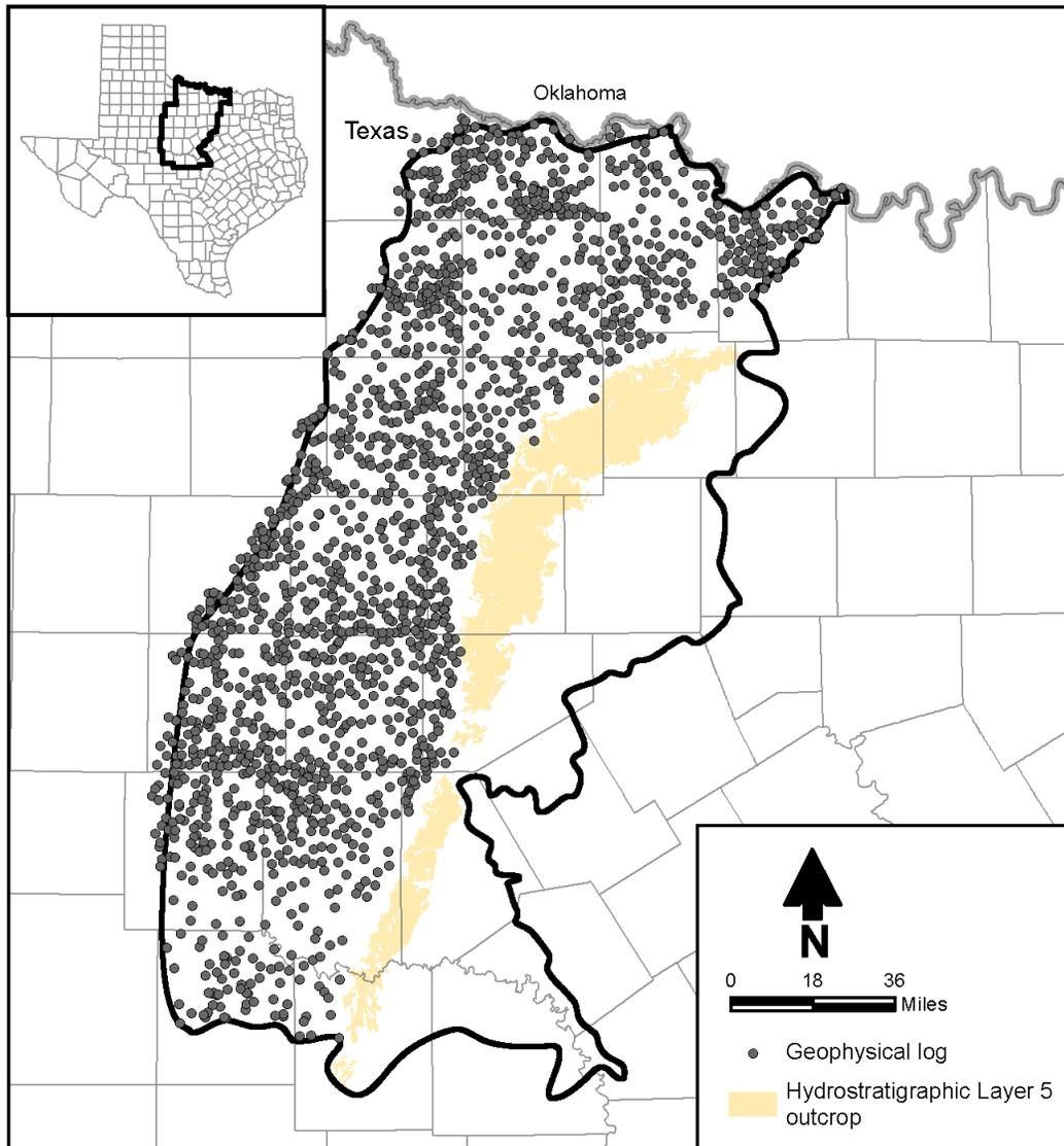
Figure 5-3. Layer 5 (Lower Cisco Group) top surface control points.
