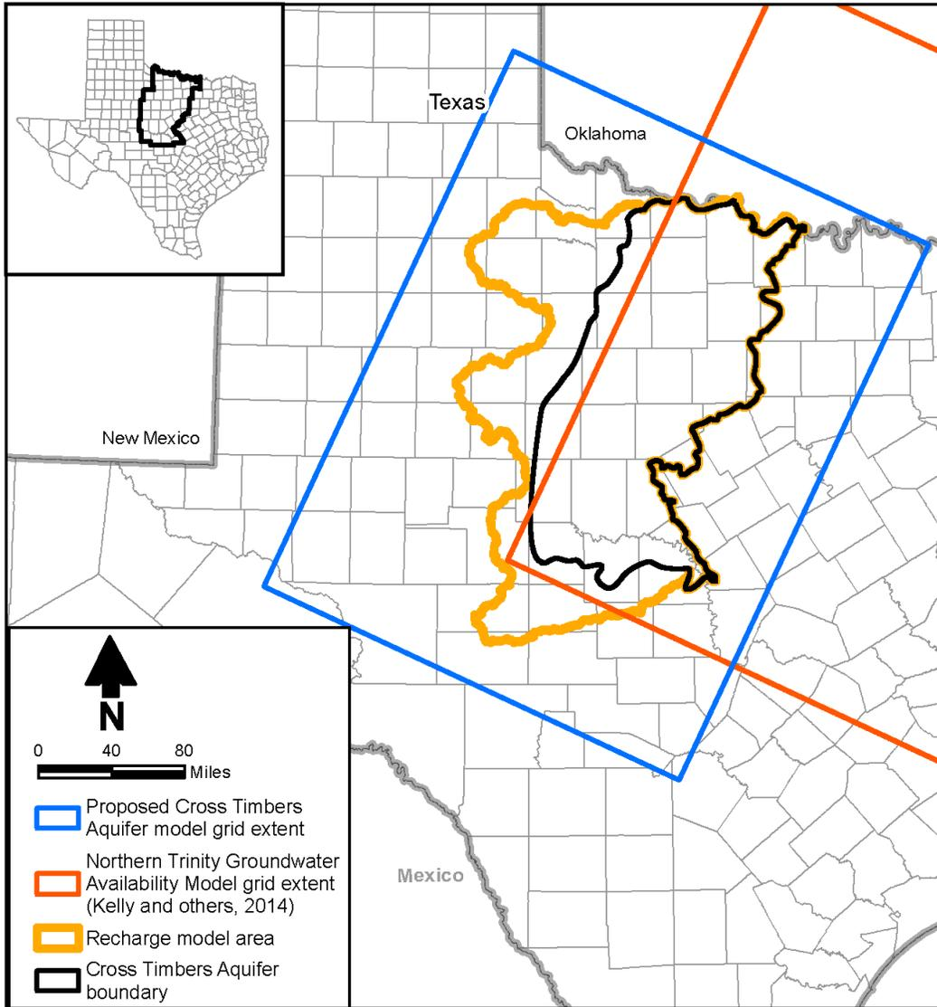
**Figure 12-3. Proposed grid for Cross Timbers Aquifer groundwater modeling.**
