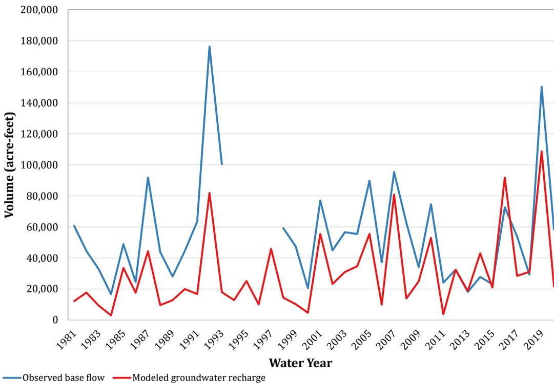
**Figure 7-7. Comparison of recharge simulation results to observed base flow for gauge 08146000 (San Saba).**
