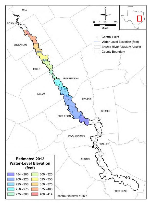
Figure 4.2.21 Estimated water-level elevation contours in feet above mean sea level in the Brazos River Alluvium Aquifer in 2012.
