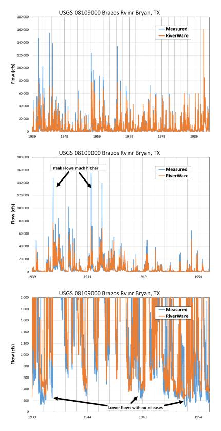
Figure 3.2.4 Actual streamflow at gage 08109000 compared to simulated streamflow.
