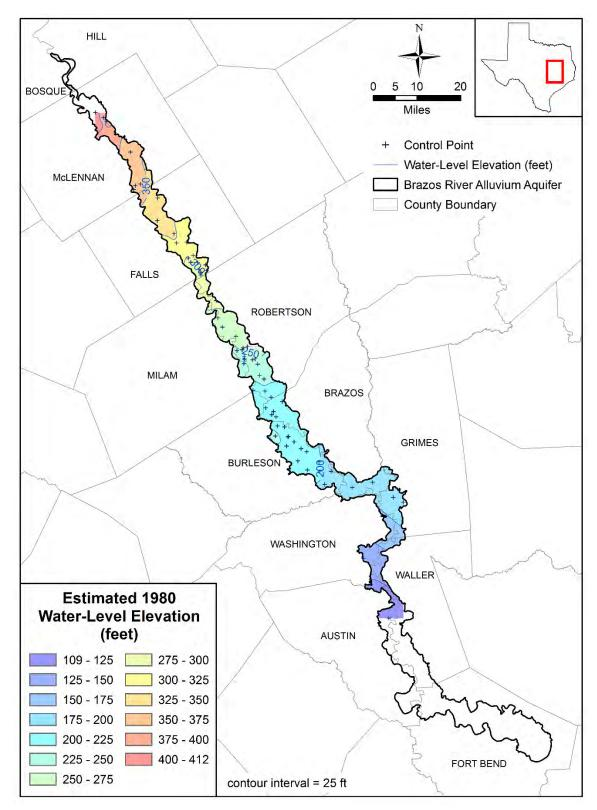
Figure 4.2.19 Estimated water-level elevation contours in feet above mean sea level in the Brazos River Alluvium Aquifer in 1980.
