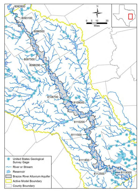
Figure 4.4.1 Rivers, streams, and United States Geological Survey stream gage locations in the vicinity of the Brazos River Alluvium Aquifer.
