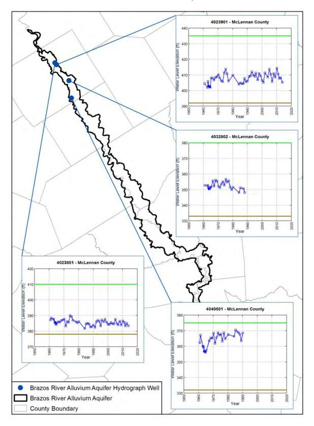
Figure 4.2.7 Select hydrographs for Brazos River Alluvium Aquifer wells located in McLennan County (TWDB, 2014f).
