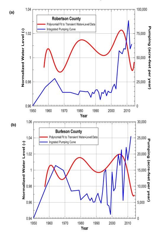
Figure 4.6.28 Comparison of integrated pumping curve and long-term water-level trend in (a) Robertson and (b) Burleson counties.
