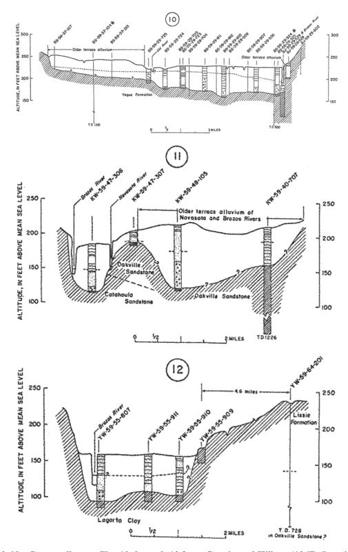
Figure 2.2.6d Cross-valley profiles 10 through 12 from Cronin and Wilson (1967) (locations given in Figure 2.2.5).
