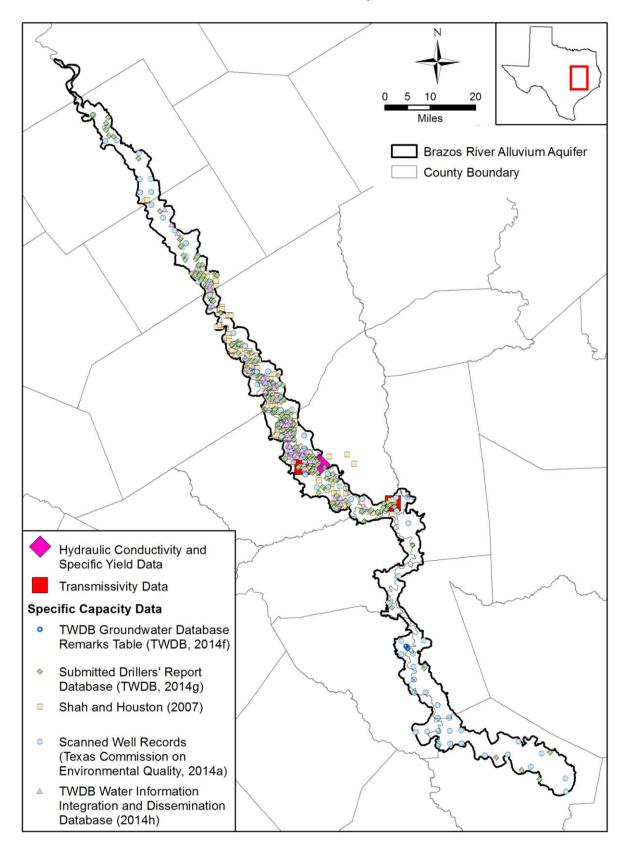
Figure 4.5.1 Available hydraulic property data for the Brazos River Alluvium Aquifer.
