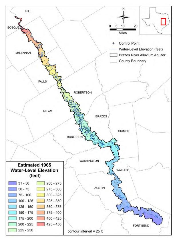
Figure 4.2.18 Estimated water-level elevation contours in feet above mean sea level in the Brazos River Alluvium Aquifer in 1965.
