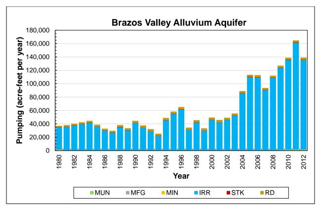
Figure 4.6.9 Bar chart of pumping from the entire Brazos River Alluvium Aquifer by use category from 1980 through 2012.
