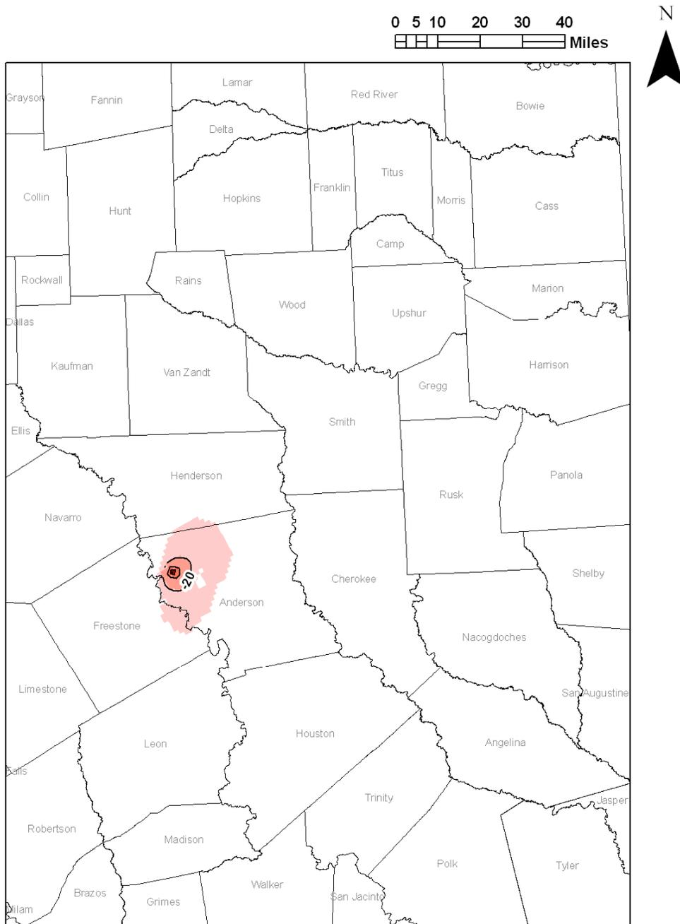
Figure 1. Water level declines in the Carrizo Aquifer after four years of pumping compared with pumping only baseline 1999 amounts. Shaded area represents declines greater than one foot and contour interval is 20 feet.
