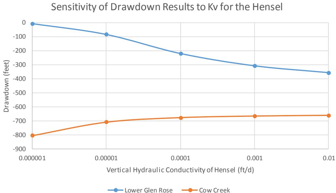
**Figure 13. Sensitivity of Cow Creek and lower Glen Rose drawdown to the vertical hydraulic conductivity of the Hensel. Assumes pumping in the EP well field of 2.47 million gallons per day. Drawdowns after 50 years shown for Bridges 1 well.**
