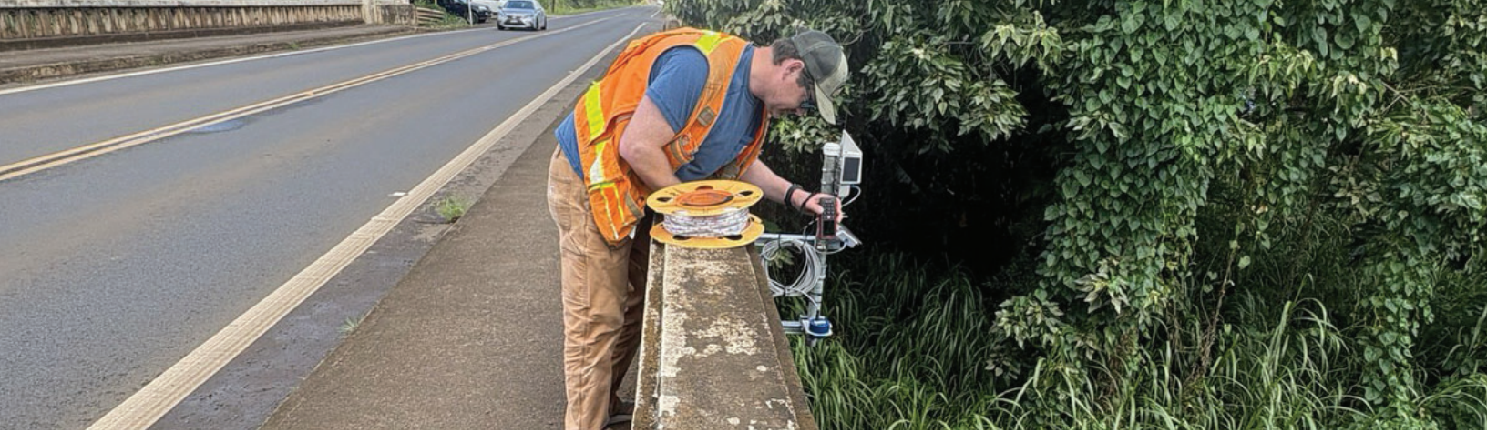
Inspecting an AWARE gage with a Geolux radar sensor in Hawaii, WEST Consultants, Inc.
