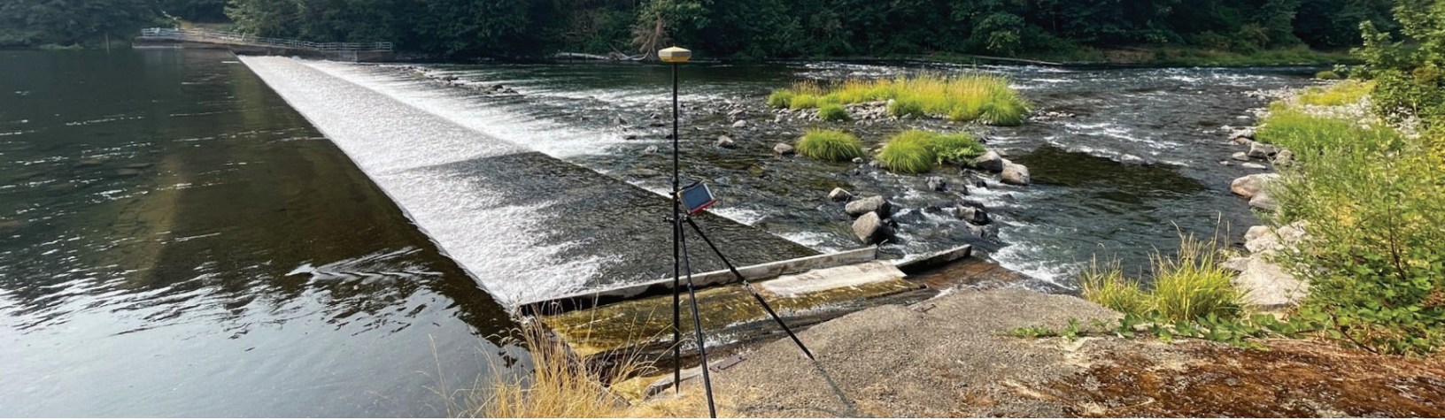
Validation of water levels on the North Santiam River using a Topcon Hiper VR RTK GNSS, Stayton, Oregon, WEST Consultants, Inc.
