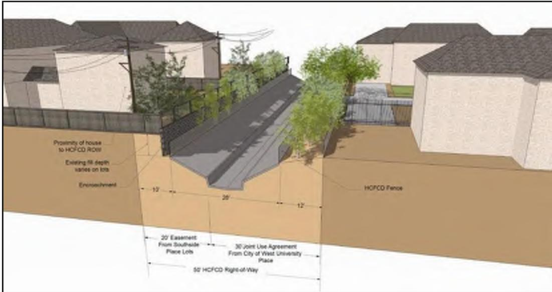
**Figure 1-1: Cross-Section Depicting Constrained Portions of Poor Farm Ditch**
