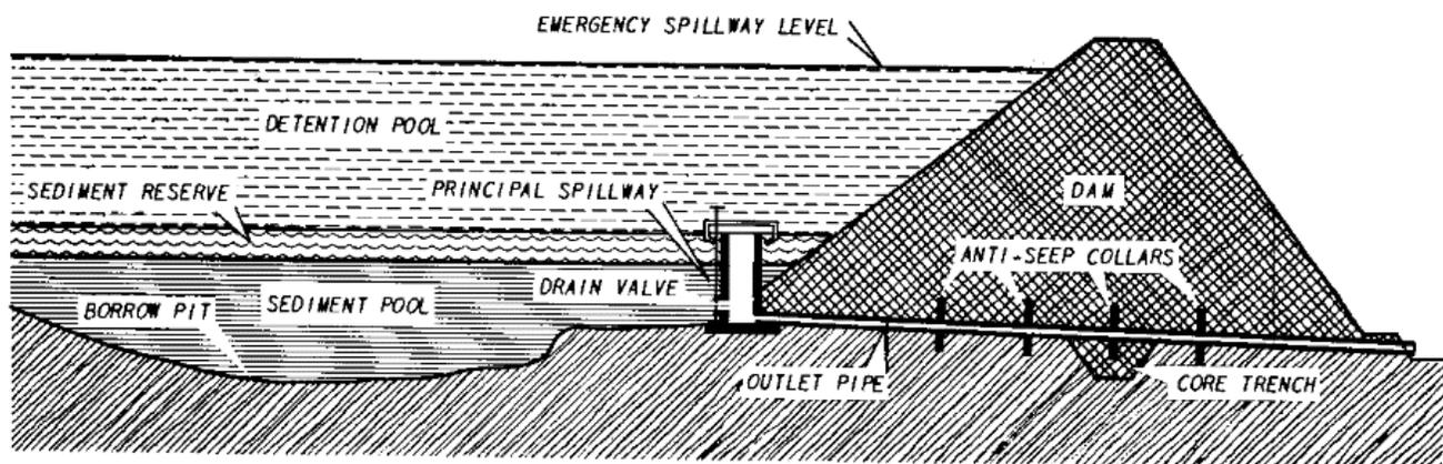
Figure 2.37 NRCS Floodwater Retarding Structures within Region 2
