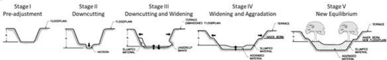
Channel enlargement is a gradual process that migrates from downstream to upstream between local base levels or hardpoints. Local base levels are features that prevent the channel from downcutting; examples may include tributary confluences, bedrock outcrops, concrete-lined channels, and culvert crossings. Geometric changes to the channel (i.e., channel enlargement) typically affect flood levels within these bounded local base levels.
