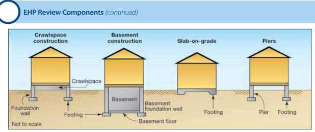
Figure 5: Examples of Foundation Types
