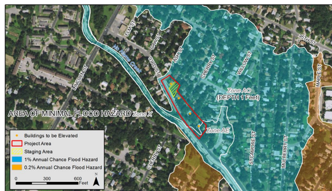
Figure 3. Example of a project site map. Map clearly shows the buildings to be elevated, the project area, the staging area, the flood zones and the BFE for the project site. The map includes a north arrow and a scale.
