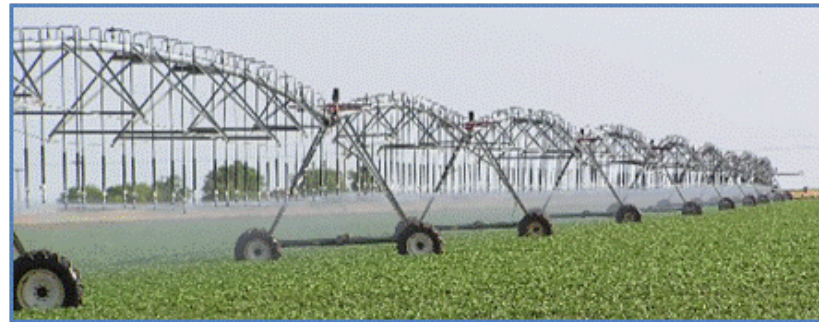
Figure 2.9. Center pivot sprinkler irrigation system equipped with mid-elevation spray applicator nozzles. Photo by Justin Mechell.
