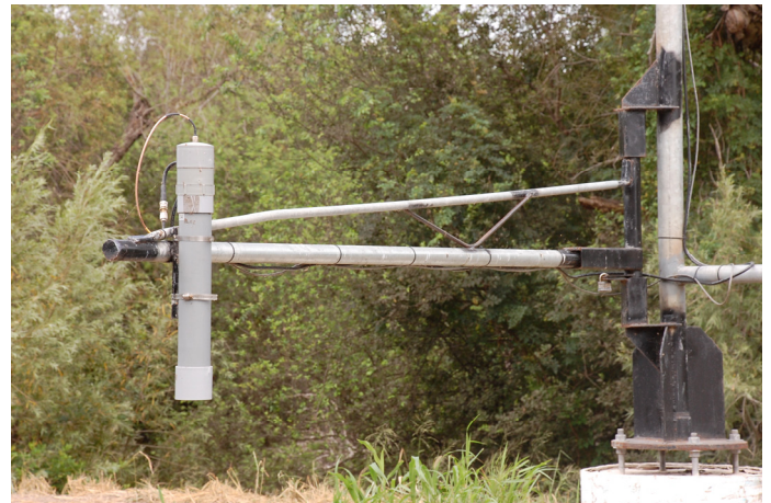
Above: Water level sensor Below: Training in auto-gate operations at the Rio Grande Center for Ag Water Efficiency
