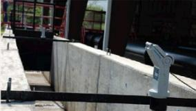
**Flow Meter Calibration Facility: Acoustic level transmitter and sharp crested weir in the 140-foot canal simulation flume.**
