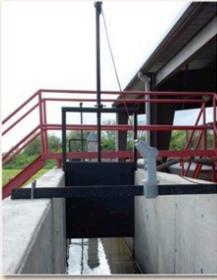
**Flow Meter Calibration Facility: Auto gate and acoustic level transmitter in the canal simulation flume.**
