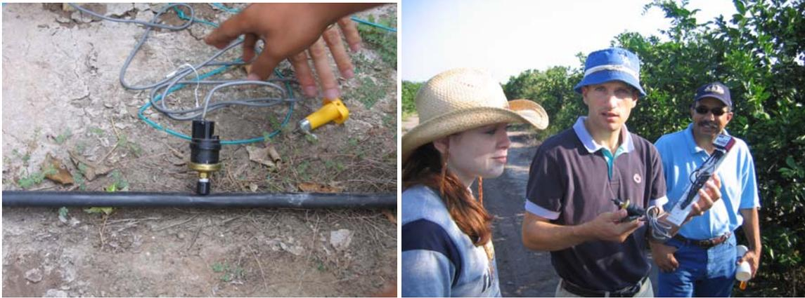
**Above:** Xavier shows pressure sensor (left; installed in drip line) to students (right).
