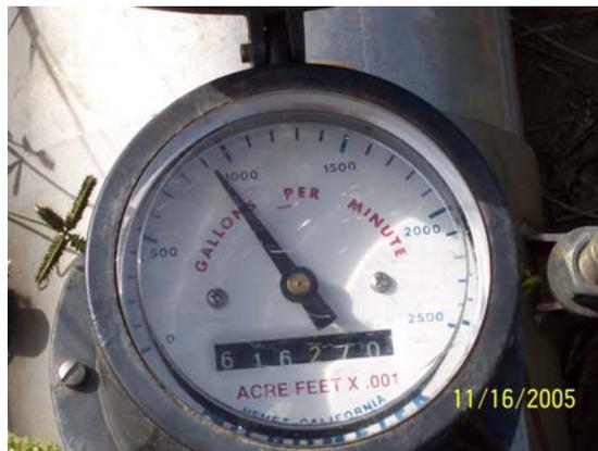
If the meter is working properly, then certain assumptions can be made, i.e. how long the field will have to be watered, depending on the total acres planted and the GPM. Pictures 6 and 7 demonstrate the progression of the watering process in a cabbage field.
