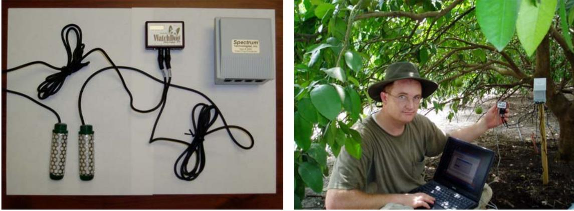
WatchDog<sup>®</sup> dataloggers equipped with WaterMark<sup>®</sup> soil moisture sensors (left) are used at various field locations to track water content within the soil profile over the growing season. Data is downloaded periodically to a computer (right) and some growers have adopted this technology as a means of irrigation scheduling.
