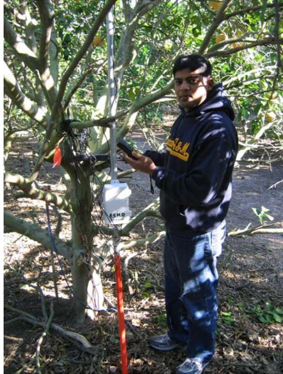
ADI collaborator Juan Ramirez has a citrus farm with mature citrus (Rio Red grapefruit, Blood navel oranges, and tangerine) under flood irrigation. Ram Uckoo, TAMUK M.S. graduate student equipped this EM-50 datalogger with 4 ECH<sub>2</sub>O soil moisture probes (left) and a rain gauge attached to the top of a metal pipe extending above the mature citrus tree canopy (left).
