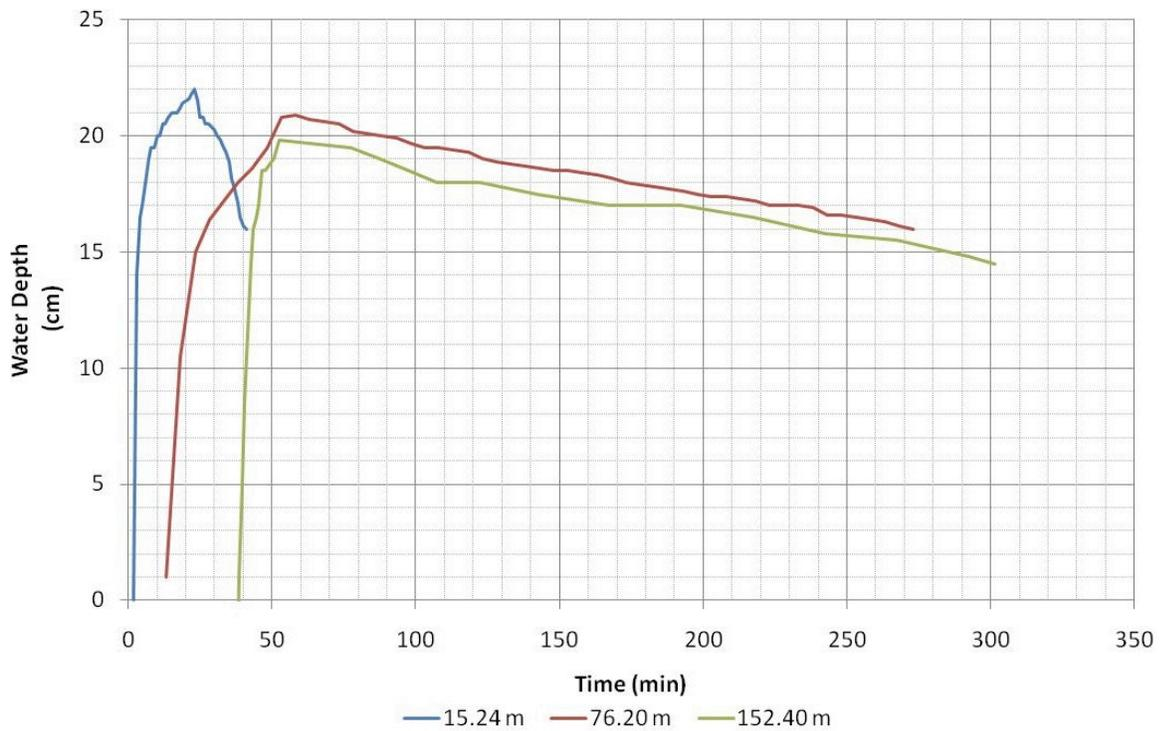
Figure 3: Hydrograph B1T1 at different location along the border 1.
