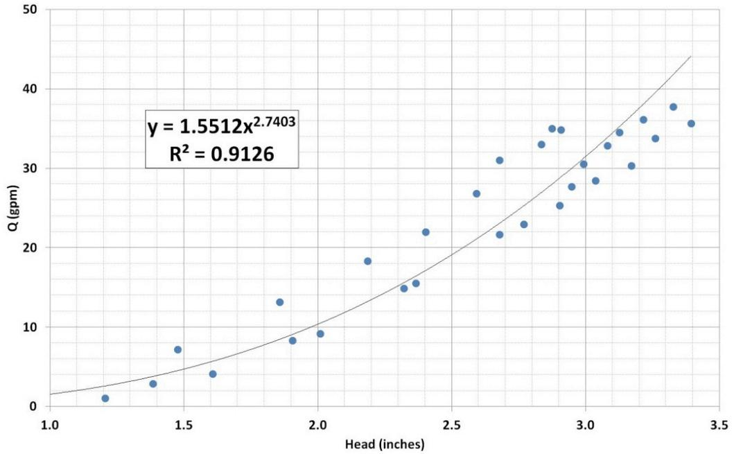
Figure 8: Circular Flume (Calibration)- Head-Discharge equation for a circular flume.
