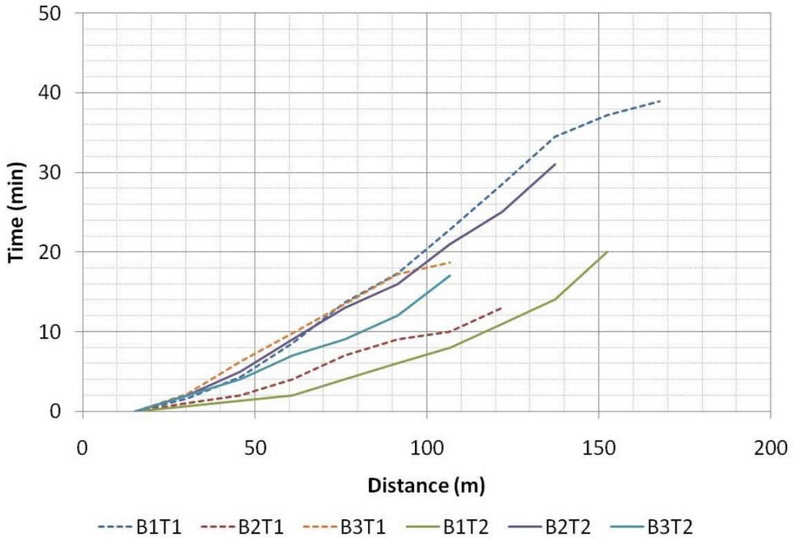
Figure 5 Advance curves for the six borders tested in the field.
