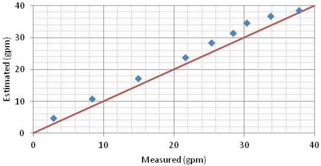
Figure 9: Measured VS Estimated discharge for flume A.
