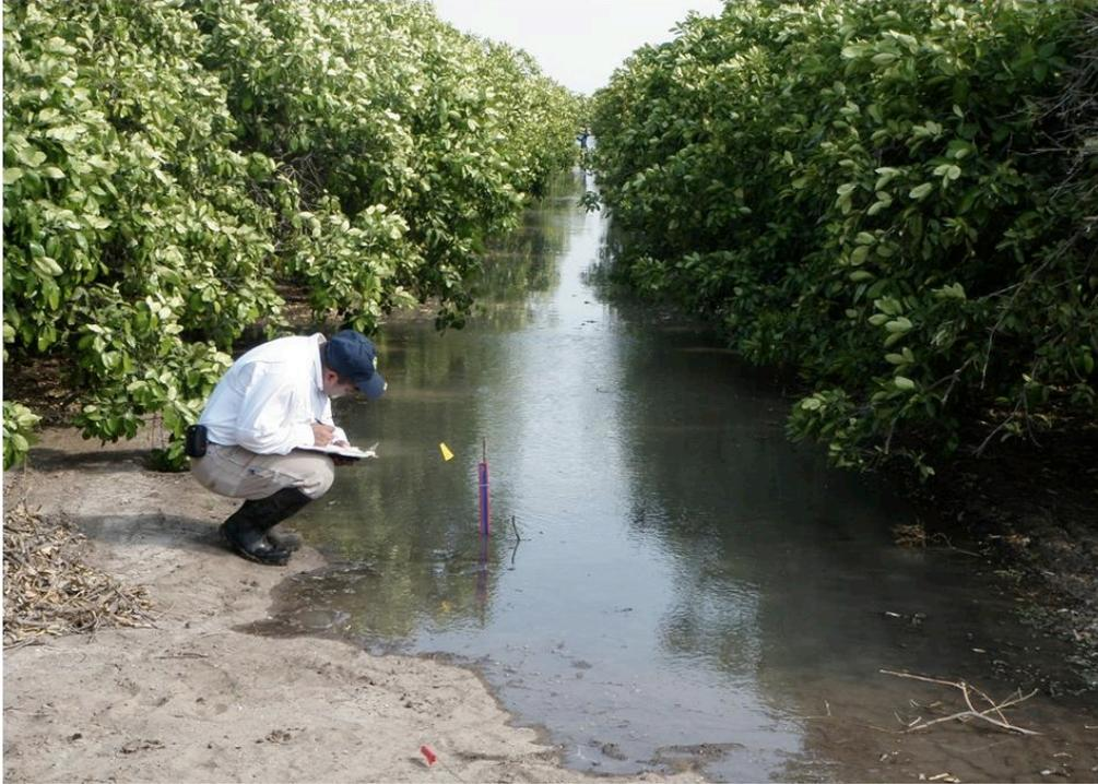
Figure 2 Water depth reading taken at the downstream end of the border.
