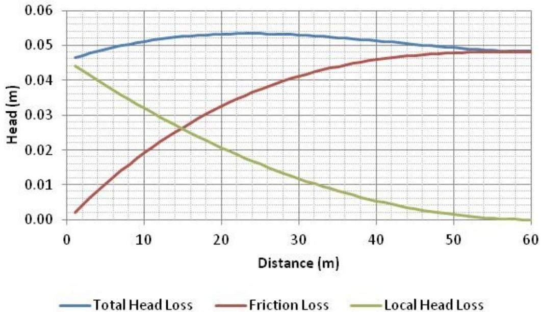
**Figure 12: Friction and local head losses in a pipe with 60 orifices.**
