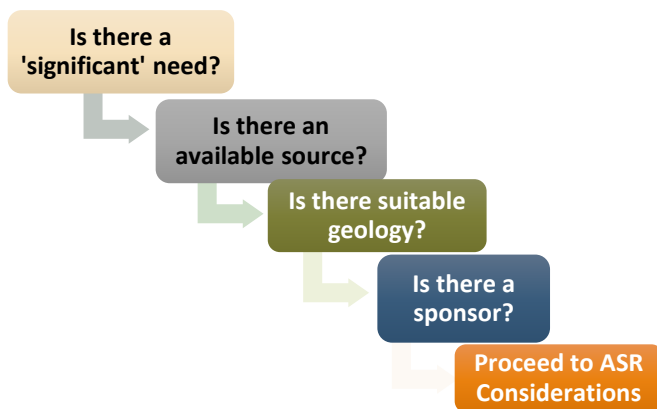
Figure 5-2 ASR Screening Process
