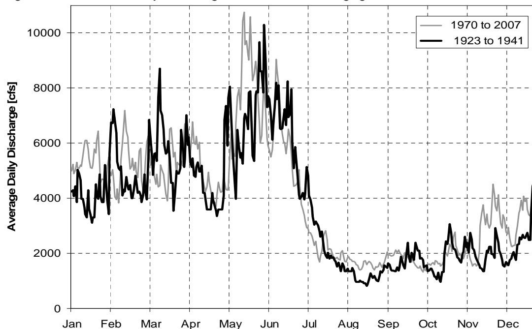
Figure 2. Median of daily discharge values for USGS gage # 08114000, Brazos River at Richmond, TX.
