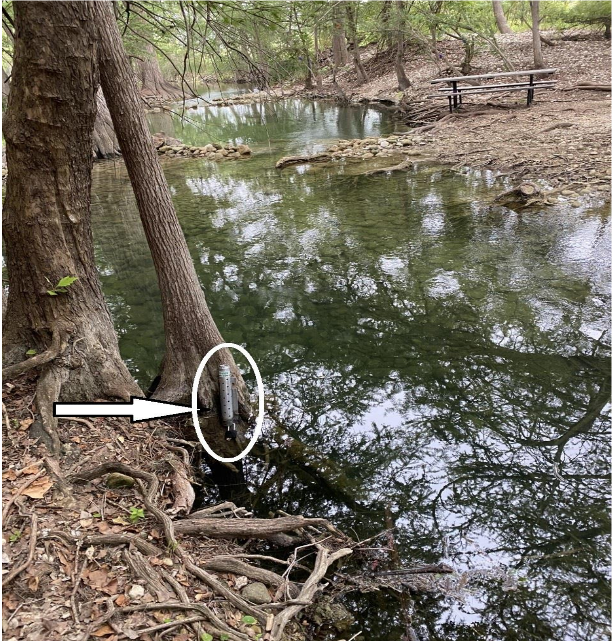
Figure 11-2, One of Five non-satellite telemetry, temporary USGS In situ Pressure Transducer – Water Level Electronic Data Loggers installed above Utopia, Tx. along the Sabinal and West Sabinal River.
