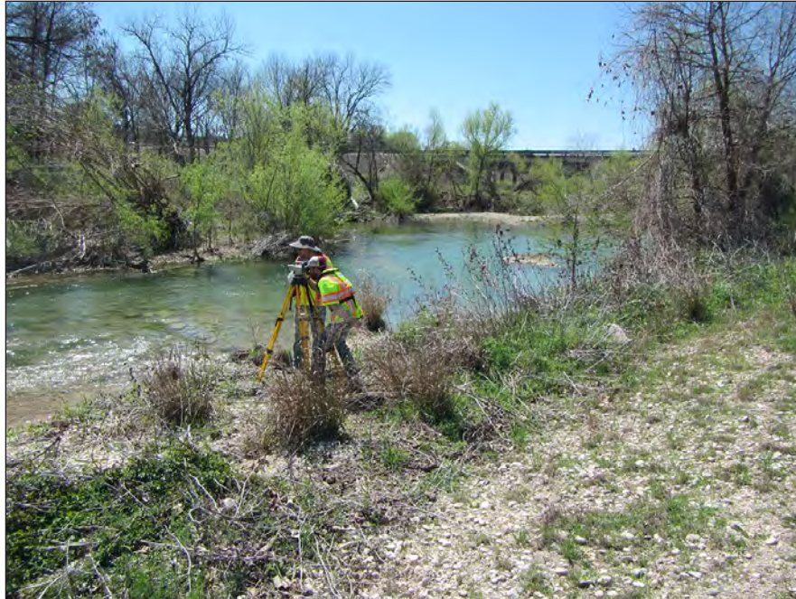
Figure 3. U.S. Geological Survey (USGS) crews performing a cross-section survey near USGS streamflow-gaging station 08178880 Medina River at Bandera, Texas. View is toward the south from the left bank of the Medina River, and Main Street bridge is shown in the background.
