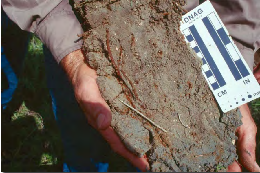
Figure 5.7. Redoximorphic concentrations of iron (red zones) along root channels are a strong indicator that this soil undergoes prolonged periods of saturation and reduction. Photo J Jacob
