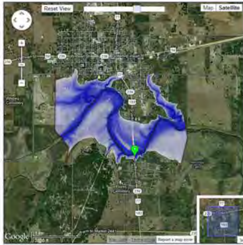
(A) The 1 in 100 year return period flood, roughly 75,000 cfs with an elevation of 143.9' (NAVD88).
