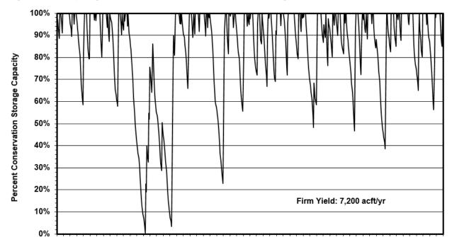
Figure 4.1-8 Spring Branch Off-Channel Reservoir Storage Trace
