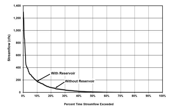
Figure 10.4-8. Frequency Comparison of Streamflow below Lake Whitney
