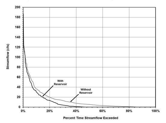
Figure 4.2-4. Brushy Creek Reservoir Streamflow Frequency Comparison
