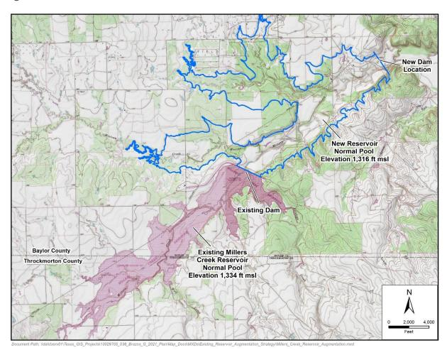
Figure 10.5-10. New Reservoir below Millers Creek Reservoir
