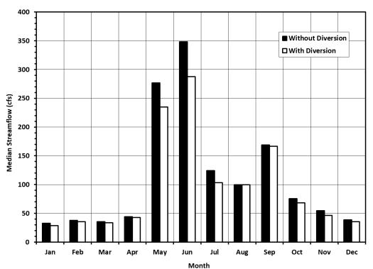
Figure 4.7-8. Brazos River Diversion Median Streamflow Comparison
