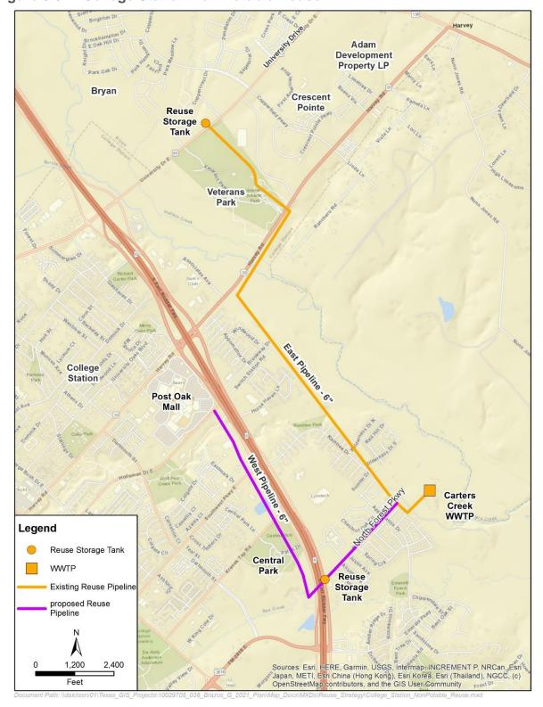
Figure 3.8-1. College Station Non-Potable Reuse
