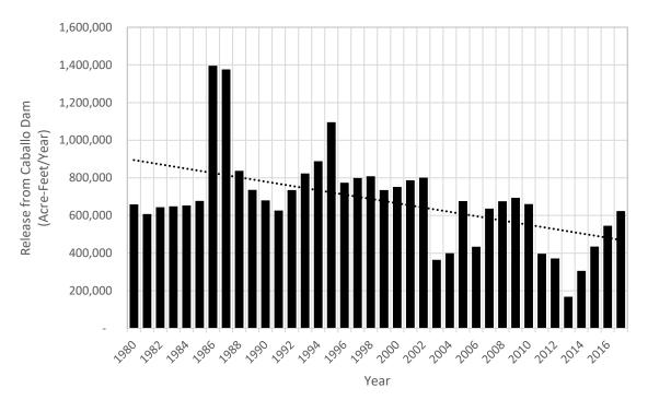
Figure 3-2. Annual Releases from Caballo Dam (Data from 1980 to 2013 is from USGS Gage 08362500 Rio Grande Below Caballo Dam, NM. Data from 2014 to 2017 is from the USBR Water Information System)
