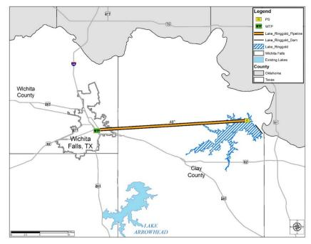
This strategy includes construction of the Lake Ringgold dam, intake pump station and a 30-mile pipeline to transport water to the City. Alternatively, the City may transport water to Lake Arrowhead for subsequent transmission to Wichita Falls. The recommend strategy supply is based on the firm yield of the reservoir based on an Excel model with extended hydrology through June 2015.
