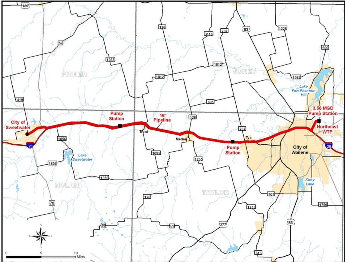
**Figure 4B.14.3-1. Treated Water Pipeline from Abilene to Sweetwater**
