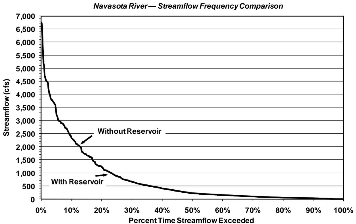
**Figure 4B.13.4-3. Peach Creek Off-Channel Reservoir and Navasota River Diversion Streamflow Comparison (Concluded)**
