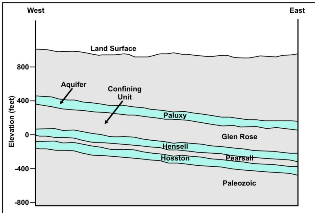
**Figure 4B.8.2-5. Hydrogeologic Profile in ASR Well Field**
