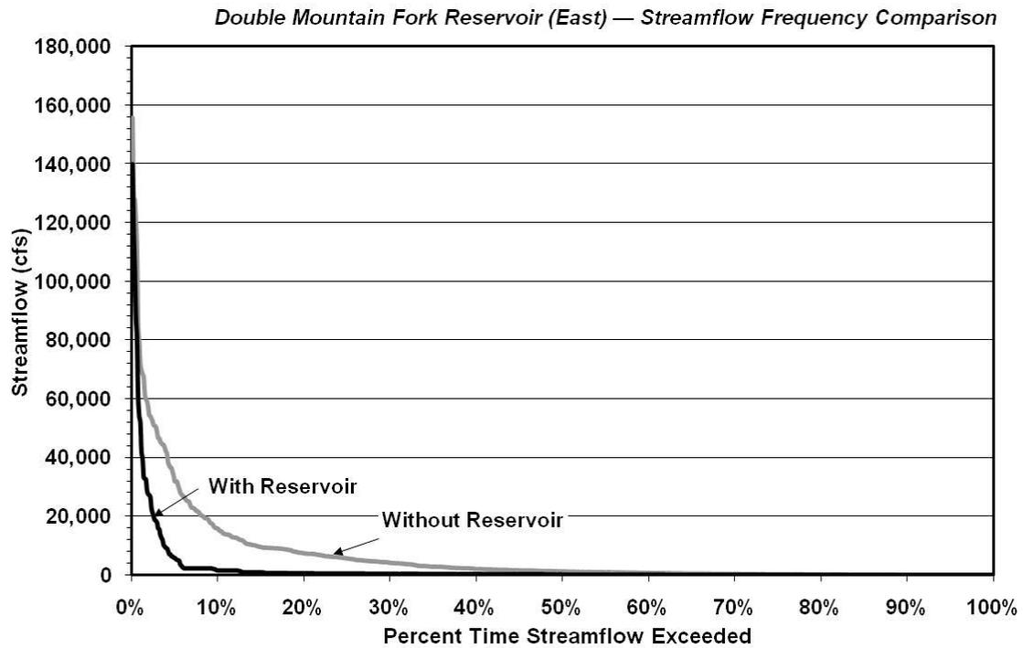
**Figure 4B.12.4-4. Double Mountain Fork Reservoir (East Site) Streamflow Comparison**
