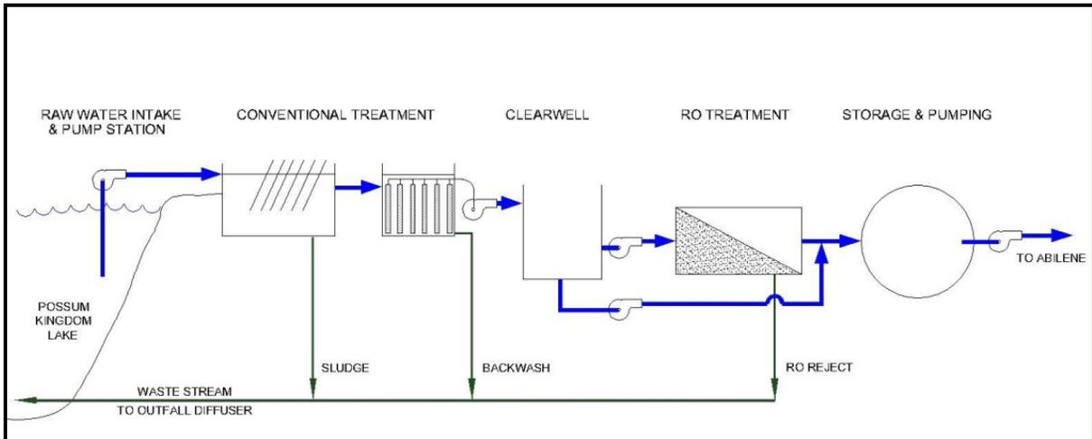
Figure 4B.14.5-2. Preliminary WTP Flow Schematic
