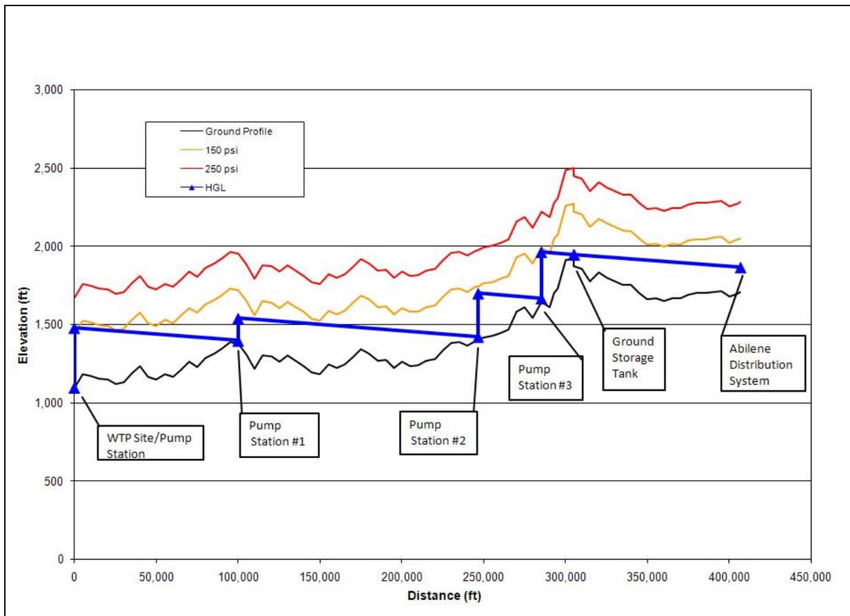
Figure 4B.14.5-7. Hydraulic Profile of Transmission System Proposed Route
