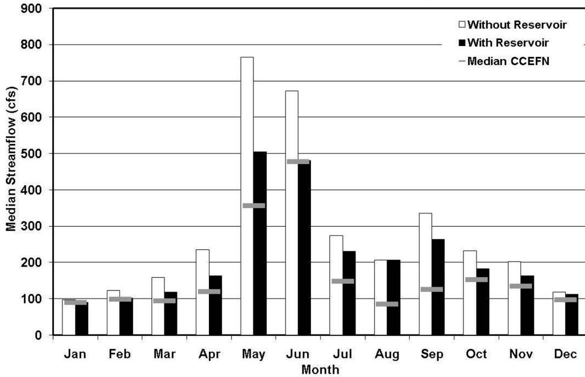
**South Bend Reservoir — Streamflow Frequency Comparison**
