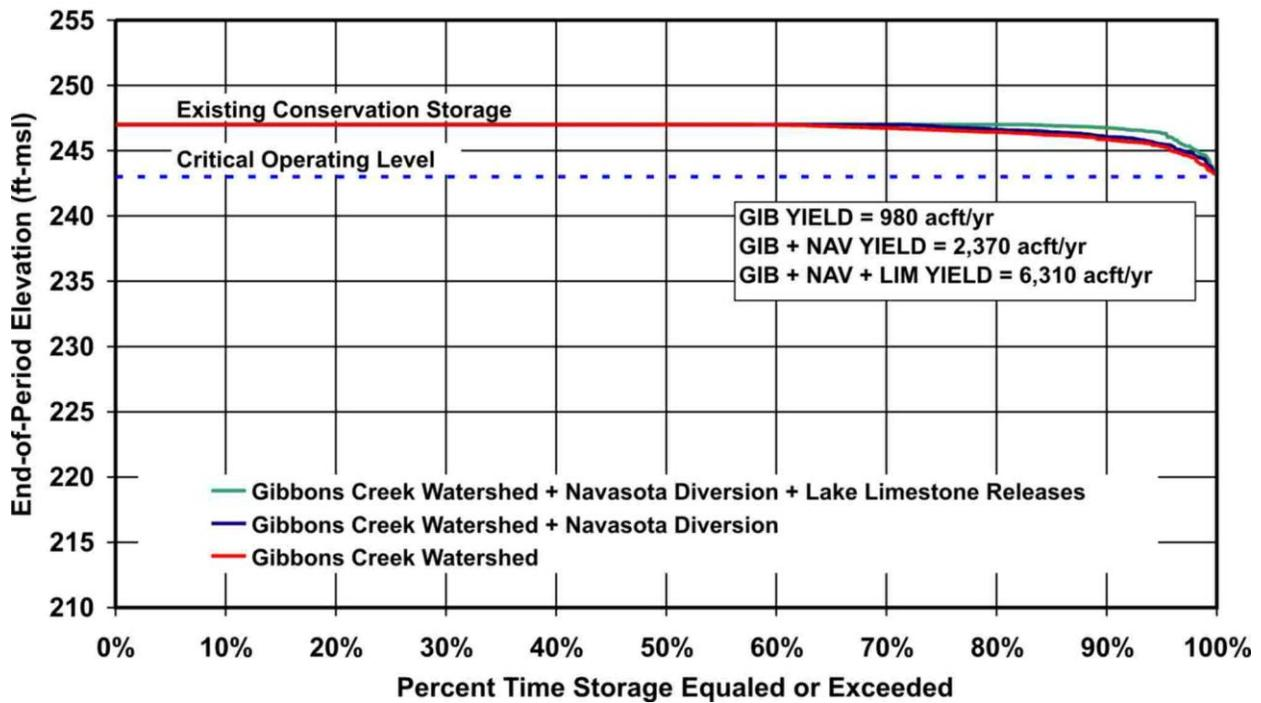
**Figure 4B.12.9-3. Monthly End-of-Period Storage for Gibbons Creek Reservoir Operating at Existing Capacity (247 ft-msl), with Critical Operating Limit Imposed**
