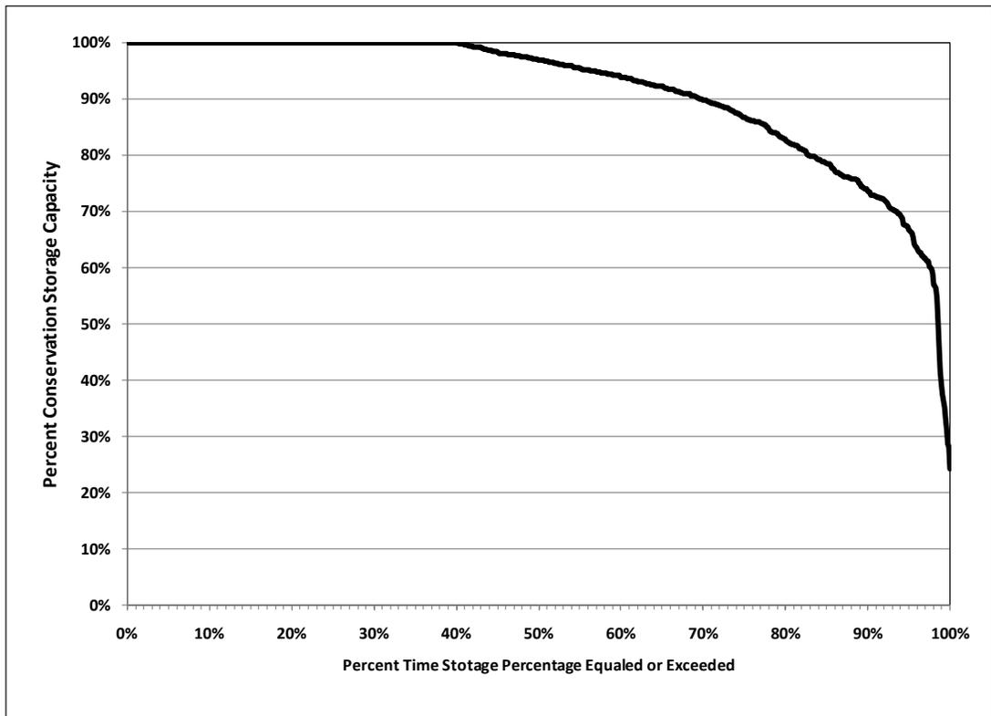
**Figure 4B.7-9. New Reservoir Storage Trace and Storage Frequency at Safe Yield with Canal Diversion**
