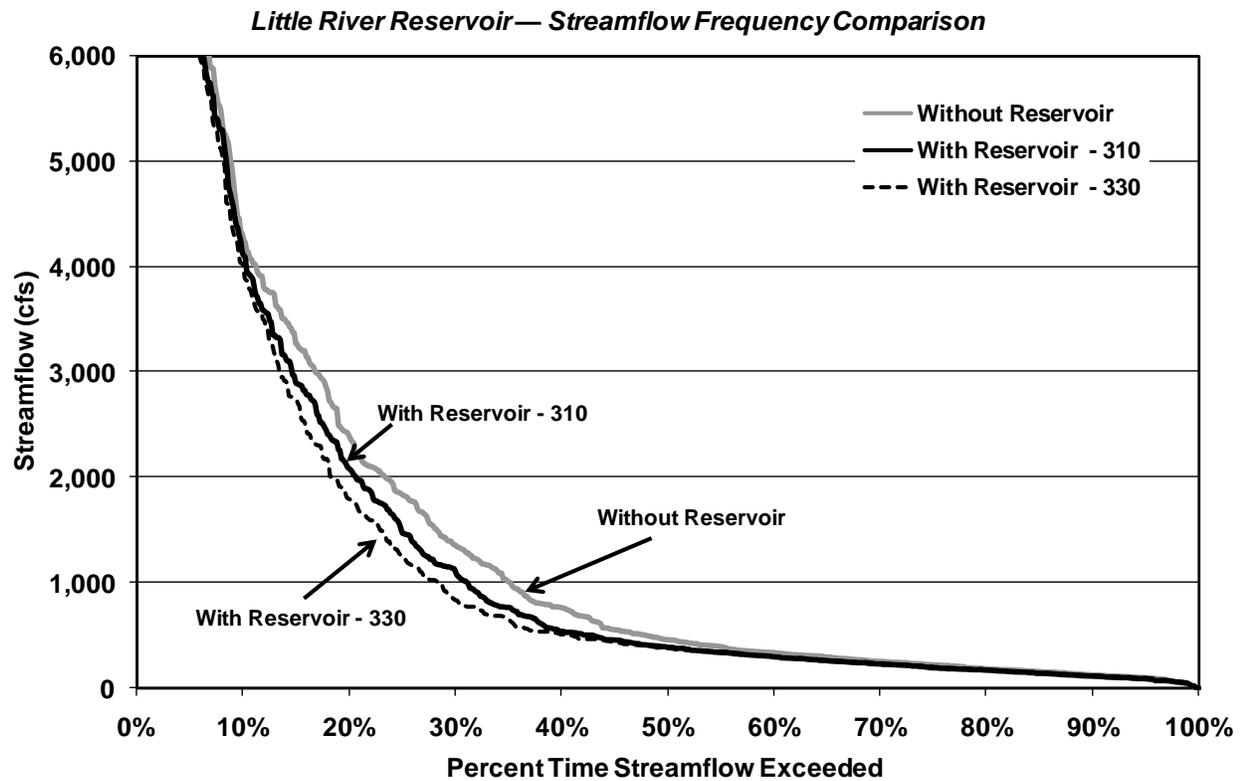
Figure 4B.12.6-3. Little River Streamflow Comparison
