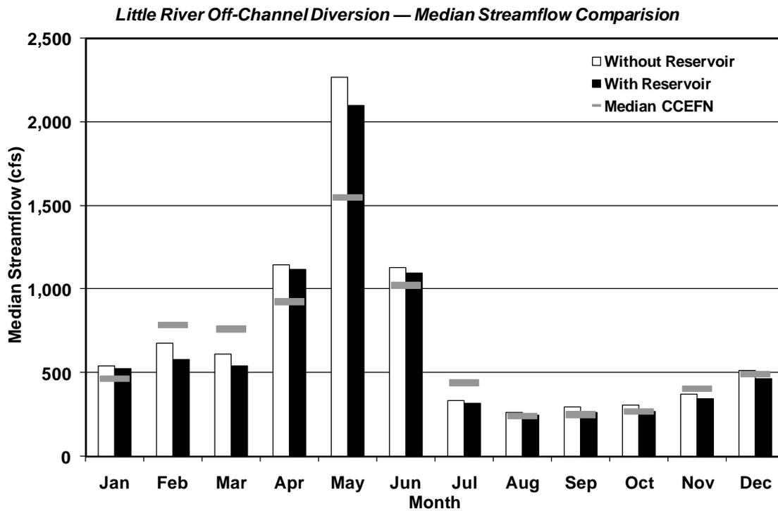
**Figure 4B.13.5-4. Little River Diversion and Reservoir Streamflow Comparison**
