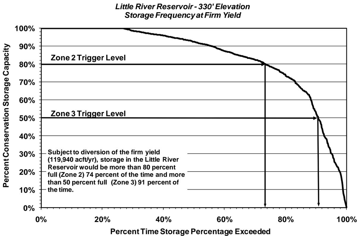
**Figure 4B.12.6-2. Little River Reservoir Storage Considerations at 310' & 330' Elevation (Concluded)**
