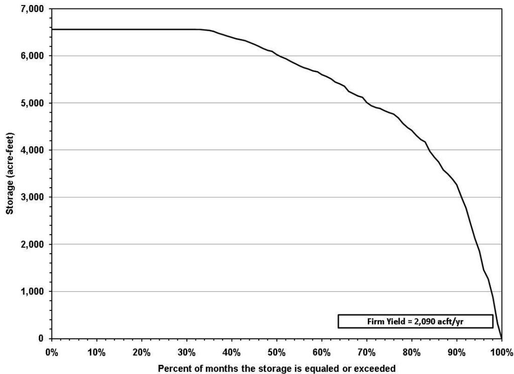
Figure 4B.12.10-3. Storage Frequency Curve for Brushy Creek Reservoir
