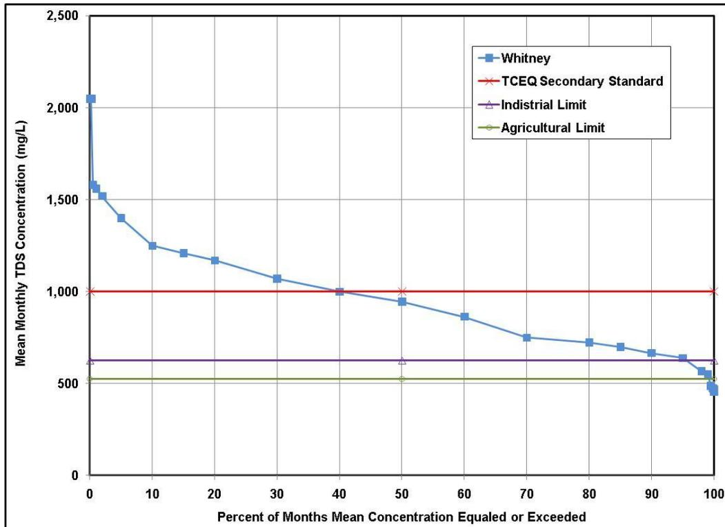
Figure 4B.19.1-5. TDS Concentration-Duration Curve at Whitney
