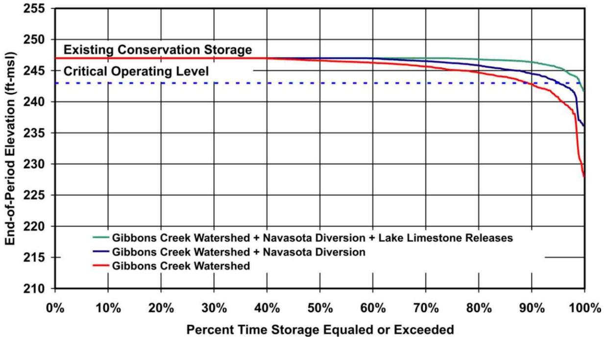
**Figure 4B.12.9-2. Monthly End-of-Period Storage for Gibbons Creek Reservoir Operated at Existing Capacity (247 ft-msl), with No Critical Operating Limit Imposed (Authorized Consumptive Demand of 9,740 acft/yr)**
