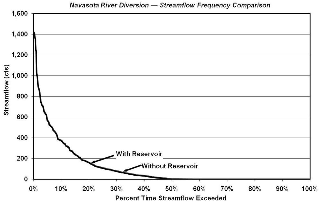
**Figure 4B.13.2-5. Groesbeck Off-Channel Reservoir and Navasota River Diversion Streamflow Comparisons**
