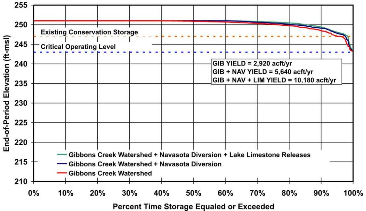
**Figure 4B.12.9-4. Monthly End-of-Period Storage for Gibbons Creek Reservoir Operated at Proposed Capacity (251 ft-msl), with Critical Operating Limit Imposed**
