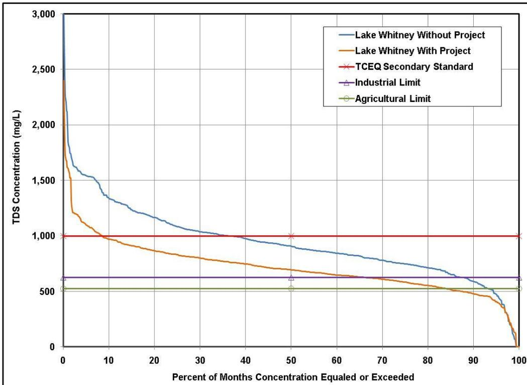
Figure 4B.19.3-5. Model-Predicted TDS Concentration-Duration Curve at Lake Whitney
