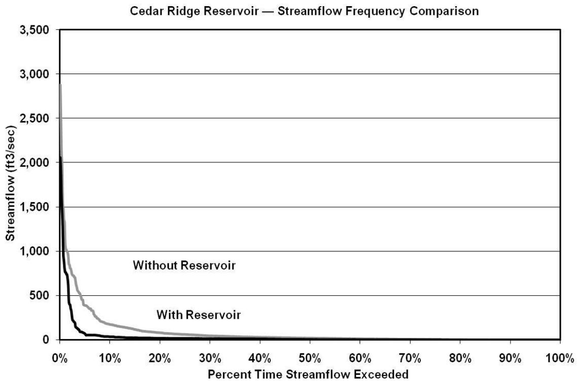
**Figure 4B.12.1-3. Cedar Ridge Reservoir Streamflow Comparisons**
