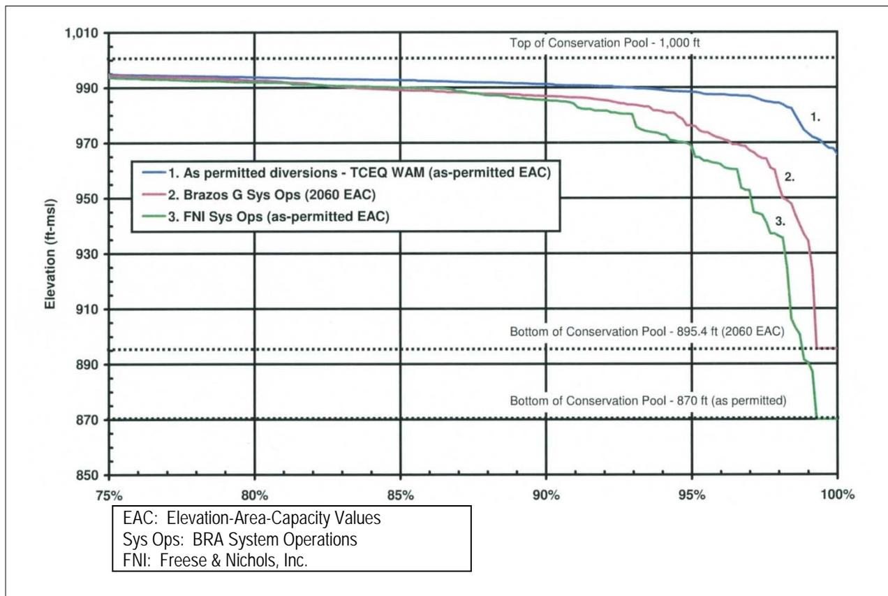
Figure 4B.14.5-5. Possum Kingdom Lake Elevation-Frequency Simulations
