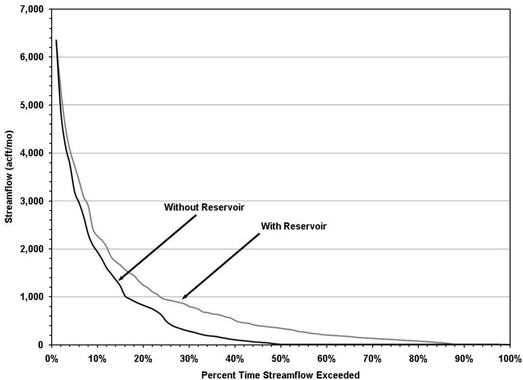
**Figure 4.12.10-4. Brushy Creek Reservoir Streamflow Frequency Comparison**
