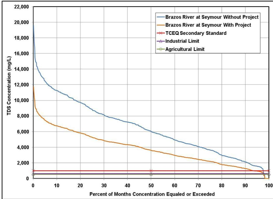
Figure 4B.19.3-2. Model-Predicted TDS Concentration-Duration Curve at Seymour
