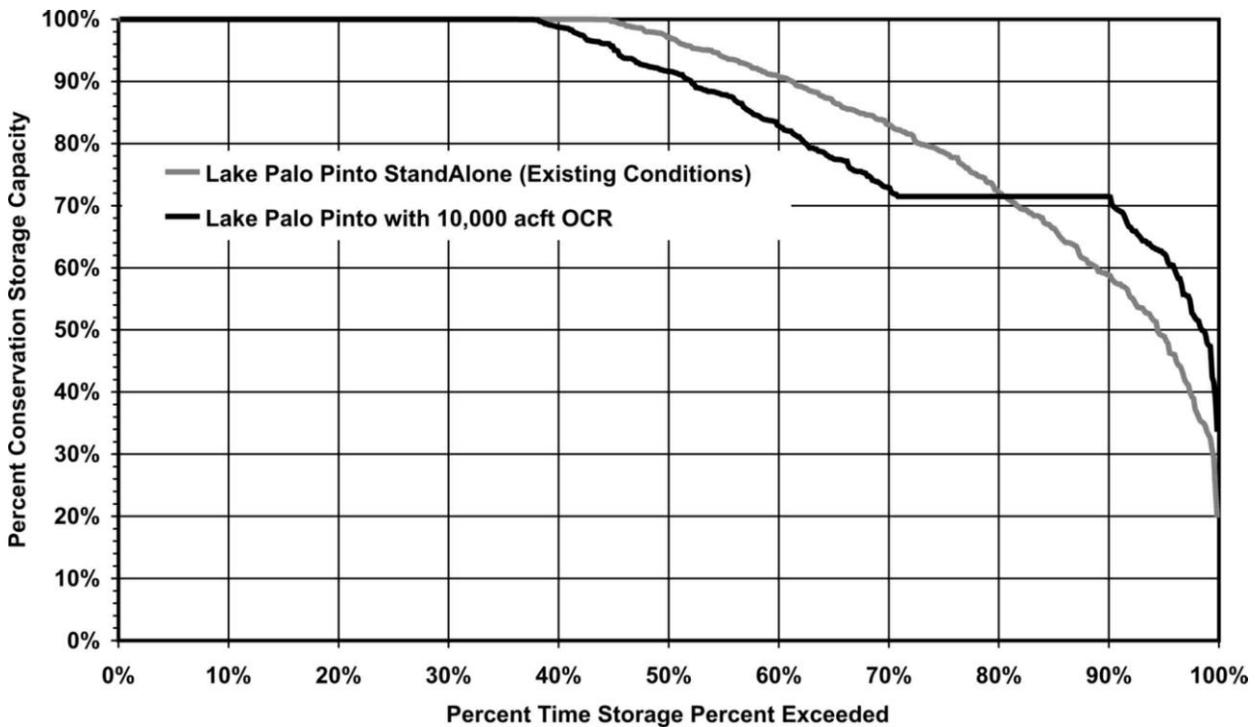
**Figure 4B.13.6-4. Comparison of Lake Palo Pinto Storage when Operated With and Without Lake Palo Pinto Off-Channel Reservoir**
