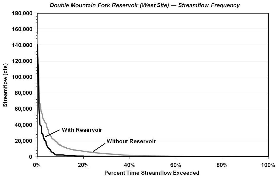
**Figure 4B.12.4-5. Double Mountain Fork Reservoir (West Site) Streamflow Comparison**
