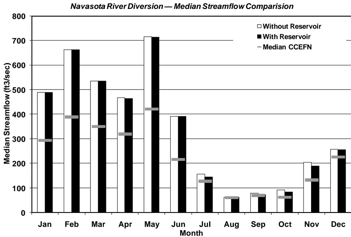
**Figure 4B.13.4-3. Peach Creek Off-Channel Reservoir and Navasota River Diversion Streamflow Comparison**
