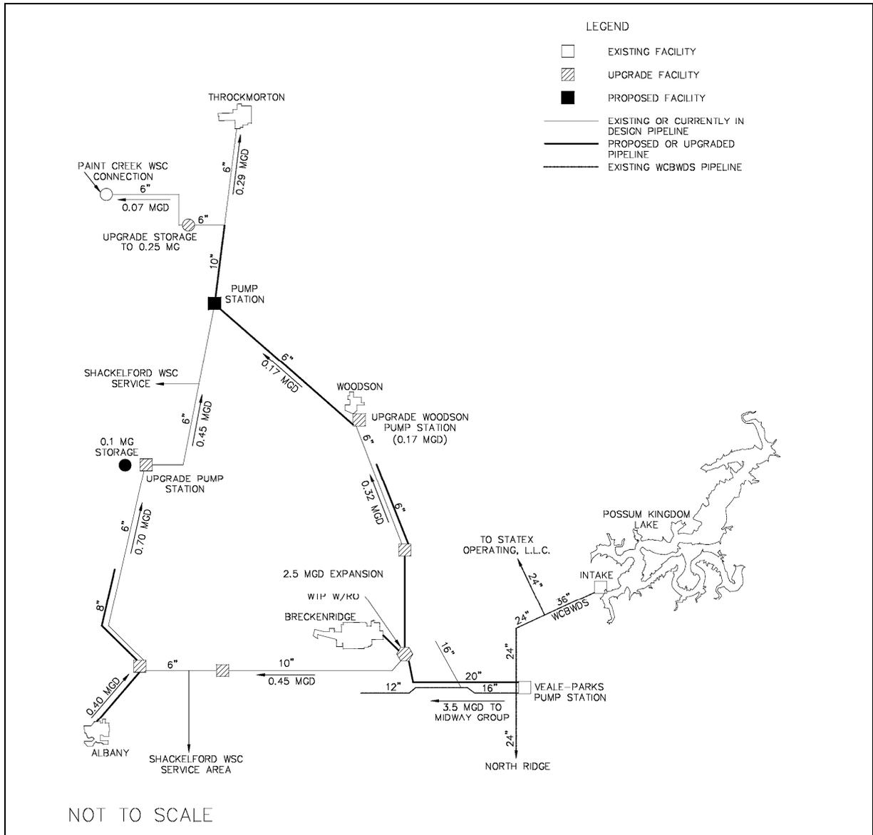
**Figure 4B.14.2-1. Schematic of Midway Group Interconnections Using the WCBWDS Facilities**
