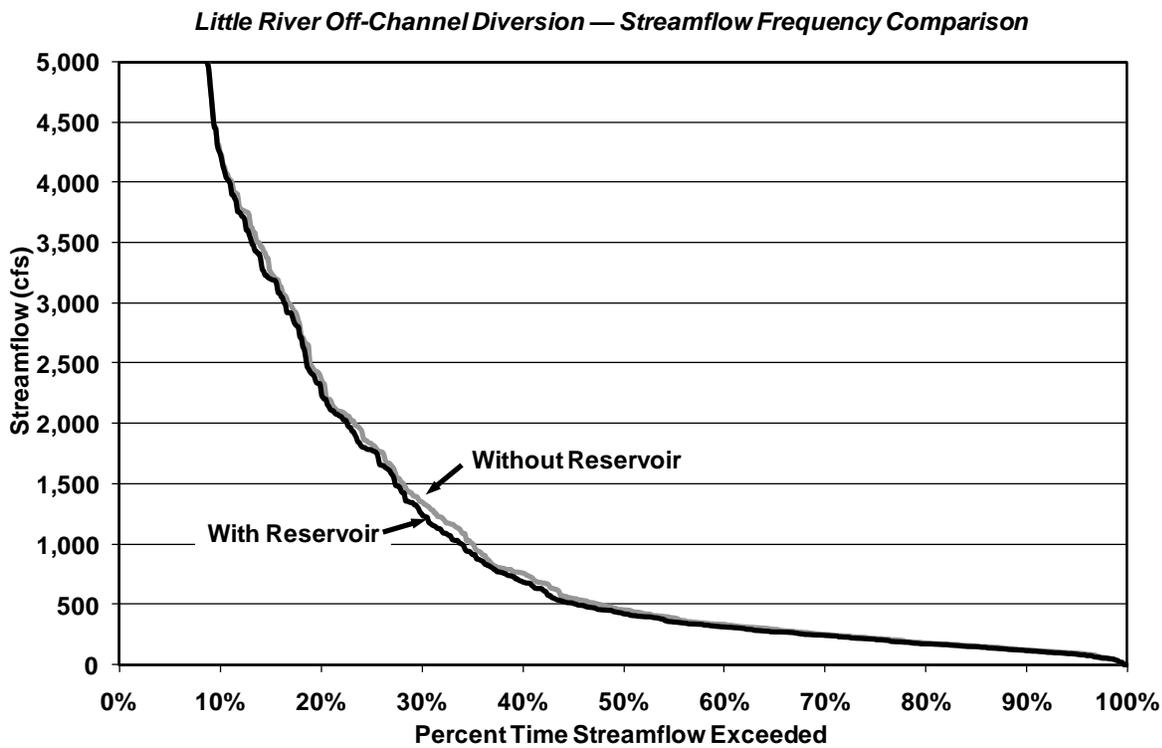
**Figure 4B.13.5-4. Little River Diversion and Reservoir Streamflow Comparison (Concluded)**
