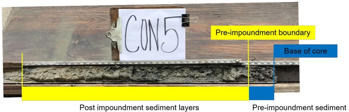
**Figure 7. Sediment core CON-5. Post-impoundment sediment layers occur in the top 37 inches of this sediment core (identified by the yellow box). Pre-impoundment sediment layers were identified and are defined by the blue box.**
