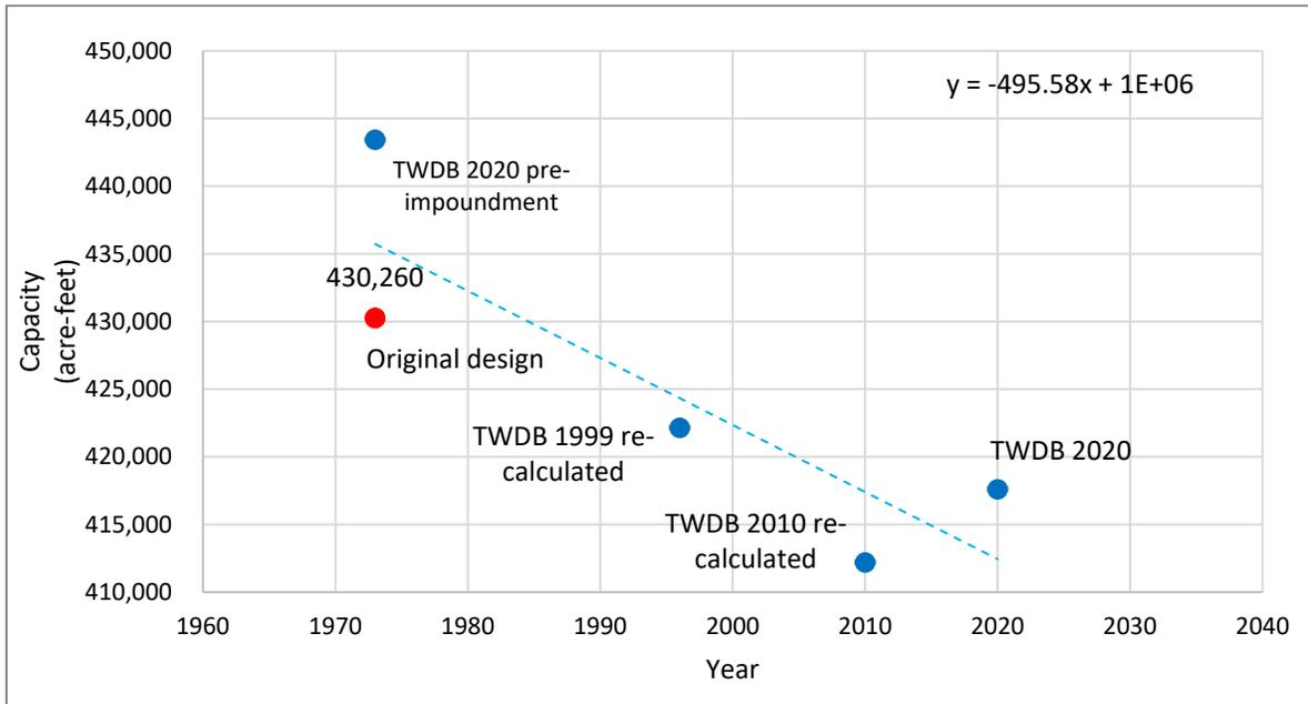
Figure 10. Plot of current and previous capacity estimates (acre-feet) at elevation 201.0 feet. Capacity estimates for each TWDB survey plotted as blue dots and other surveys as red dots. The blue trend line illustrates the total average loss of capacity through 2020.
