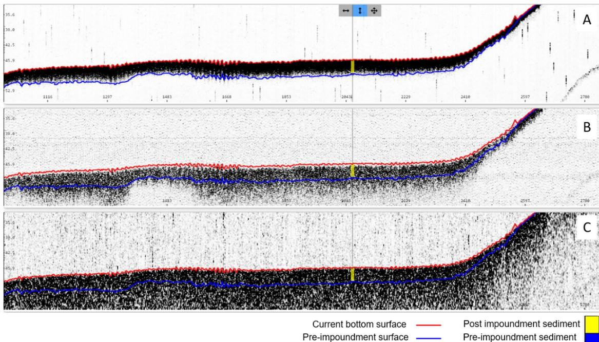
**Figure 8. Sediment core sample CON-5 compared with acoustic signal returns. A) 208 kHz frequency, B) 50 kHz frequency, and C) 12 kHz frequency.**
