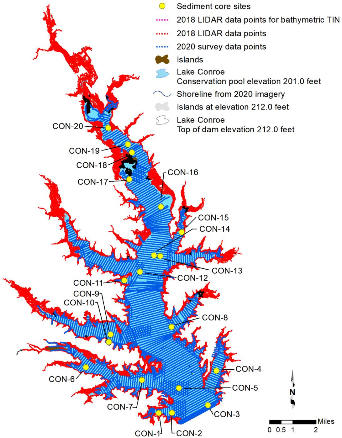
Figure 2. 2020 TWDB sounding data (blue dots), sediment coring locations (yellow circles), and 2018 LIDAR data (red dots).
