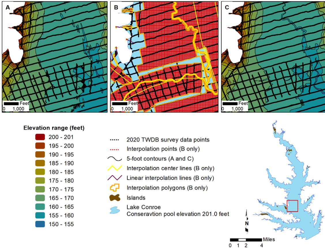
**Figure 3. Anisotropic spatial interpolation as applied to Lake Conroe sounding data; A) bathymetric contours without interpolated points, B) sounding points (*black*) and interpolated points (*red*), C) bathymetric contours with interpolated points.**
