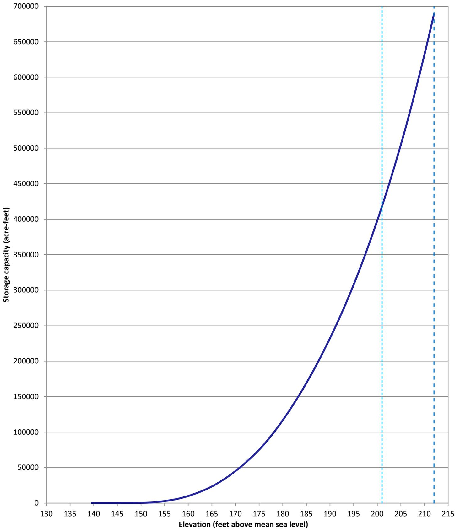
— Total capacity 2020    - - - Conservation pool elevation 201.0 feet    - - - Top of dam elevation 212.0 feet
