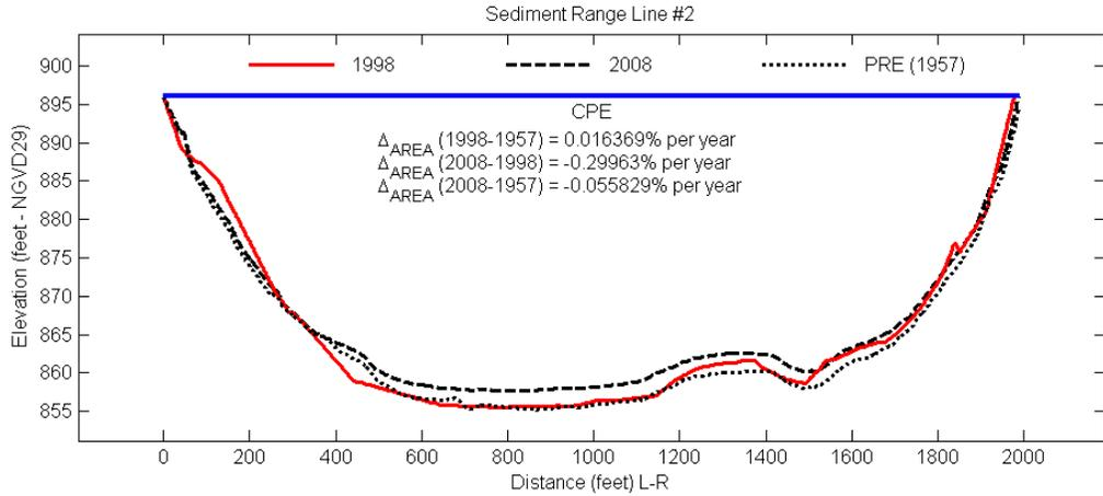
Figure E3– Cross-section plots for sediment range line #2 for Lake Weatherford.
