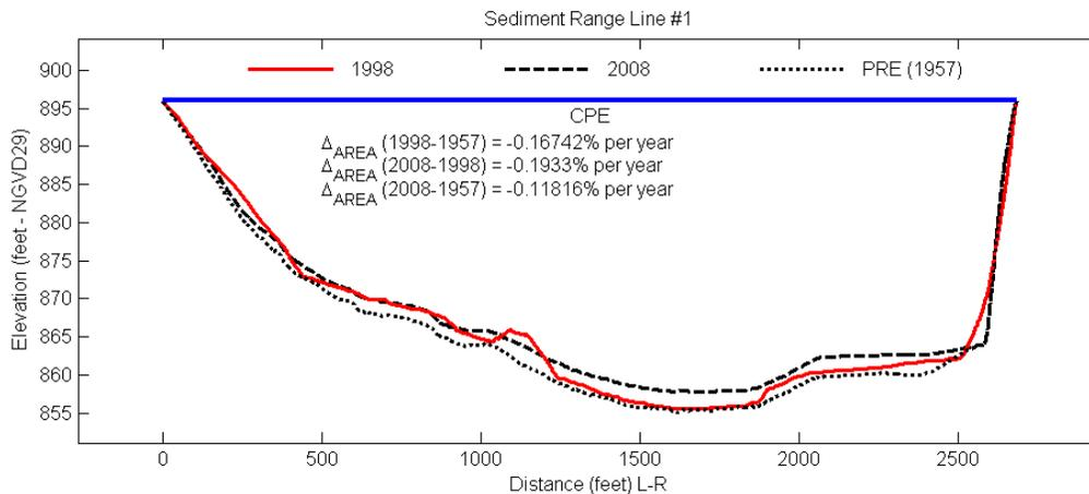
Figure E2– Cross-section plots for sediment range line #1 for Lake Weatherford.
