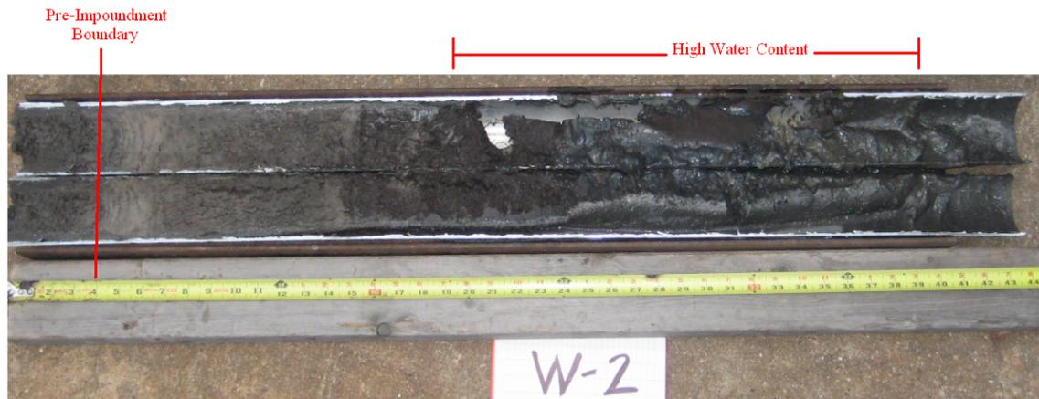
Figure D2 – Sediment Core W-2 from Lake Weatherford, showing the pre-impoundment boundary 4 inches above the base of the core (left). The pre-impoundment boundary is marked by the change in soil structure below and above the area 4” up from the core base. Above 20” from the core base, the sediment moisture content is extremely high.
