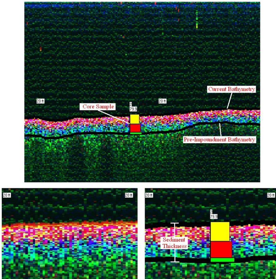
Figure D3 – DepthPic and core sample use in identifying the pre-impoundment bathymetry.
