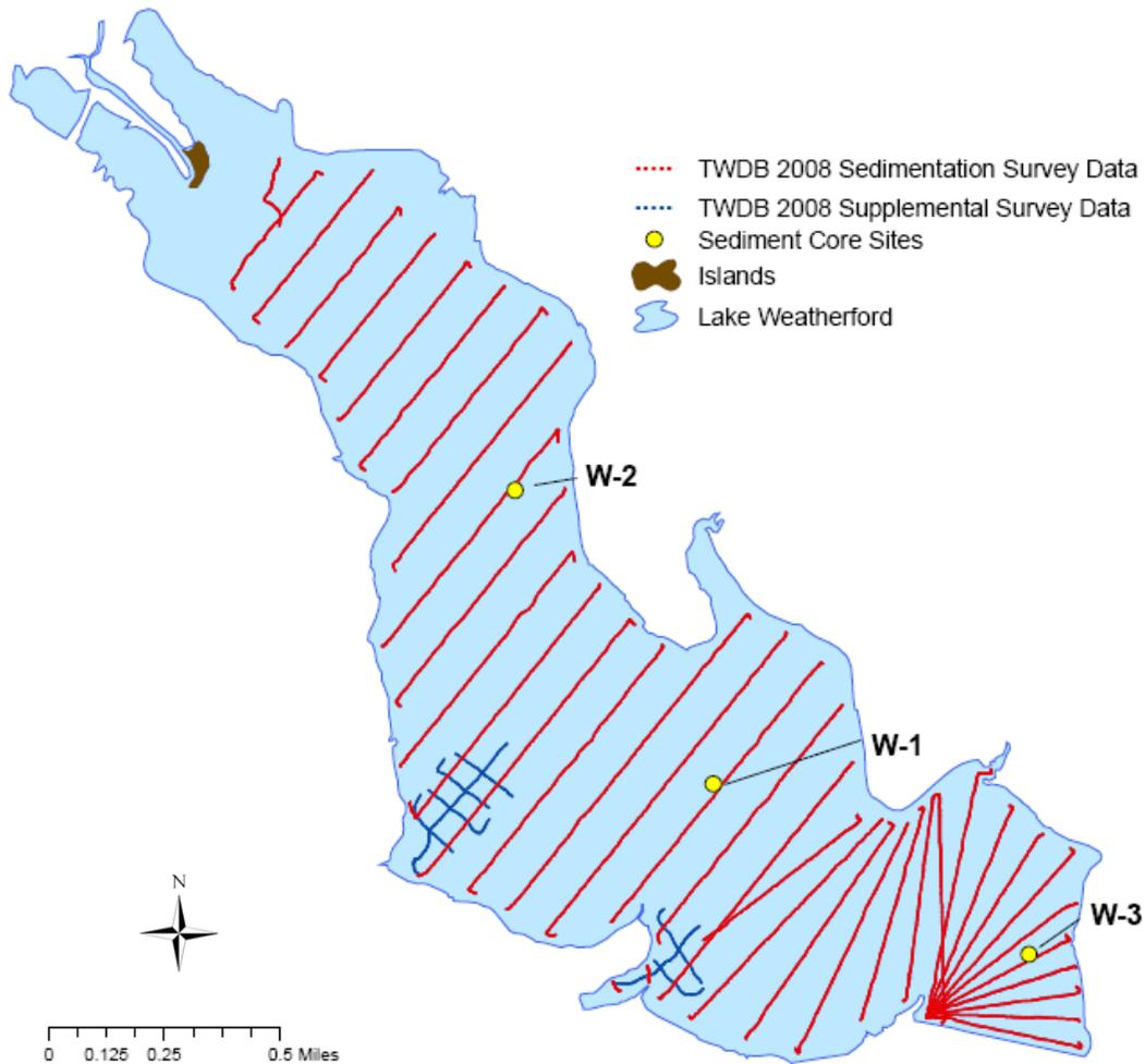
*Figure D1 – TWDB 2008 survey data points for Lake Weatherford. Sounding data used in assessing sediment content are shown in red.*
