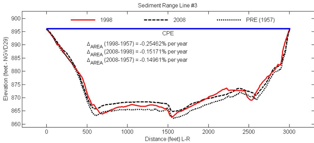
Figure E4– Cross-section plots for sediment range line #3 for Lake Weatherford.
