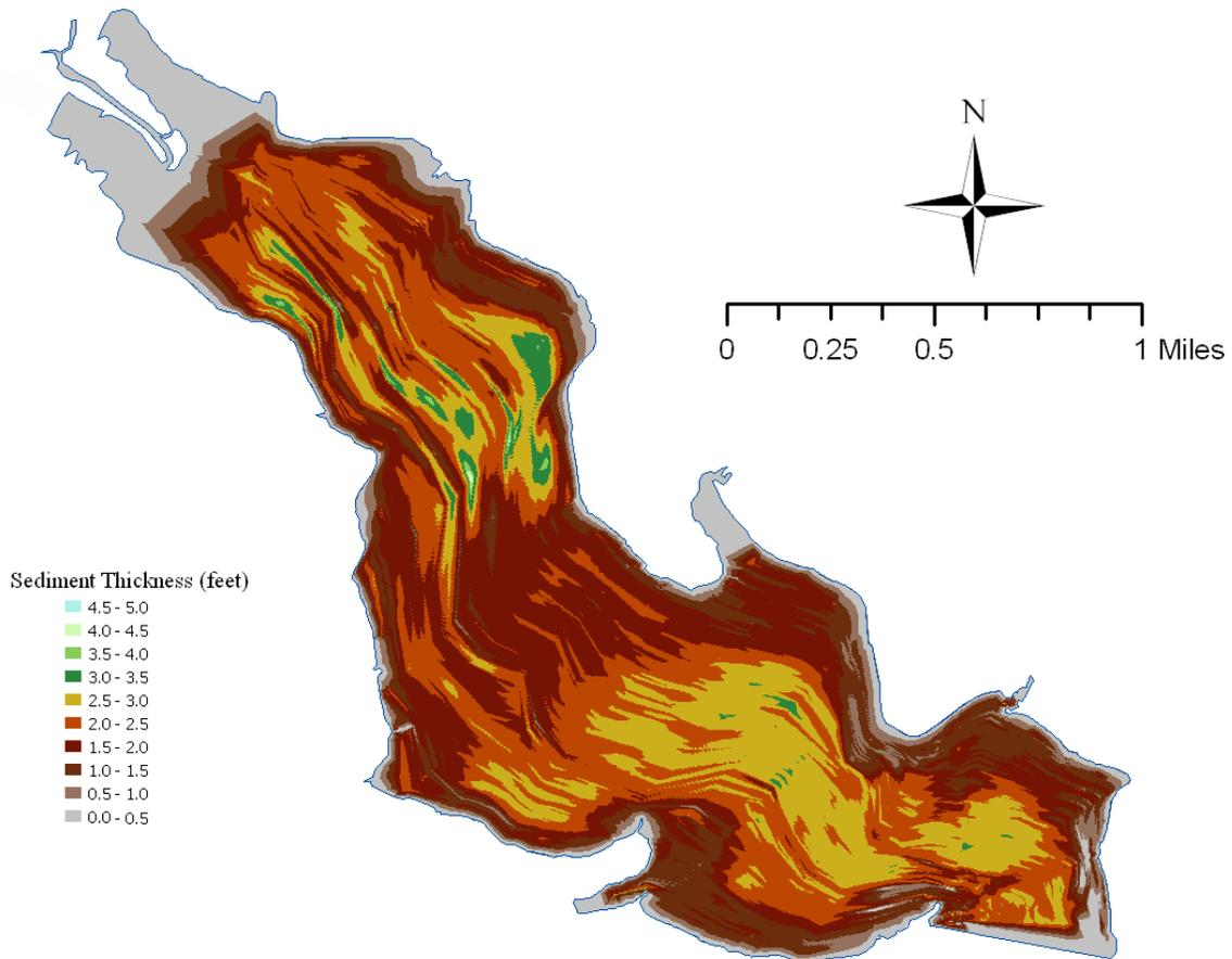
Figure D4 - Sediment thicknesses in Lake Weatherford derived from multi-frequency sounding data.
