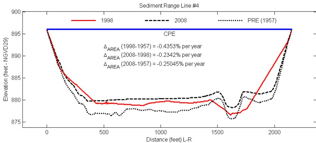
Figure E5– Cross-section plots for sediment range line #4 for Lake Weatherford.
