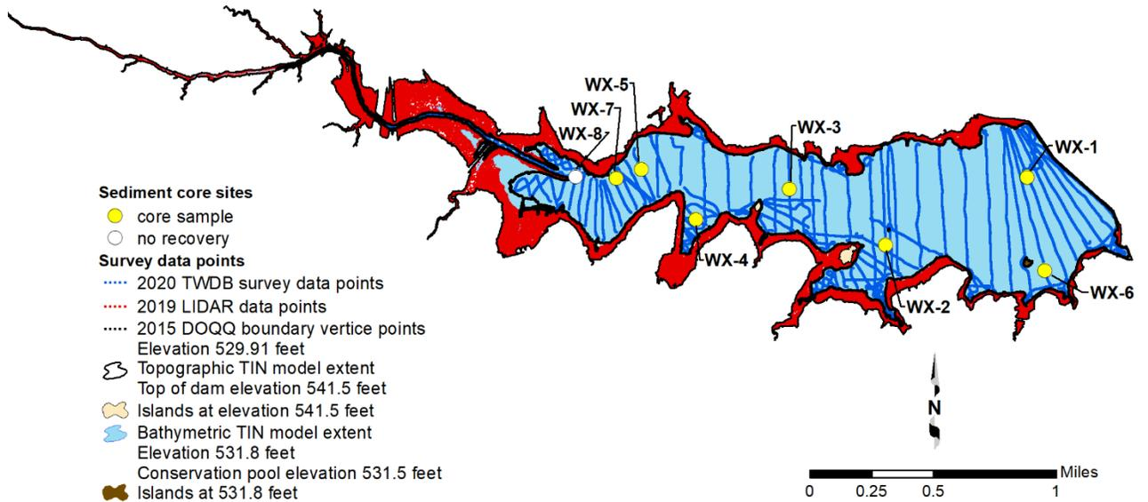
Figure 2. 2020 TWDB sounding data (blue dots), 2019 LIDAR data (red dots), and sediment coring locations (yellow circles).
