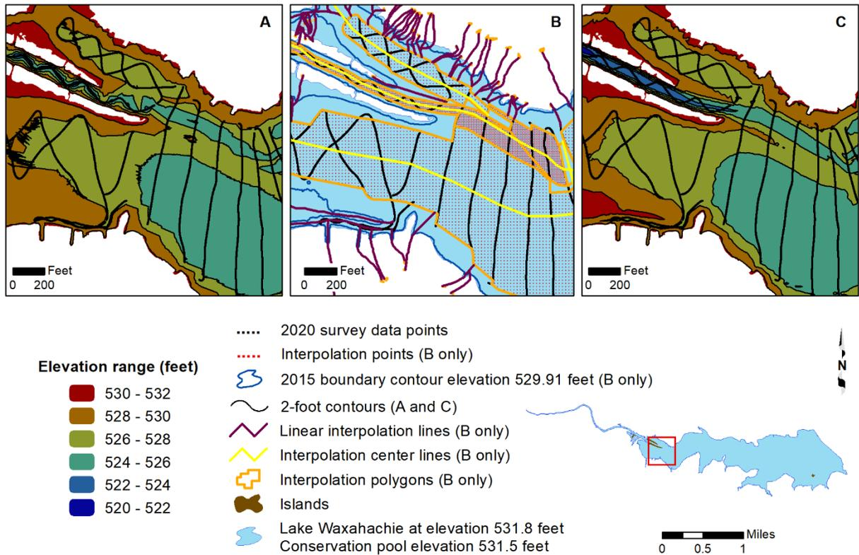
**Figure 3. Anisotropic spatial interpolation and linear interpolation as applied to Lake Waxahachie sounding data; A) bathymetric contours without interpolated points, B) sounding points (*black*) and interpolated points (*red*), C) bathymetric contours with interpolated points.**
