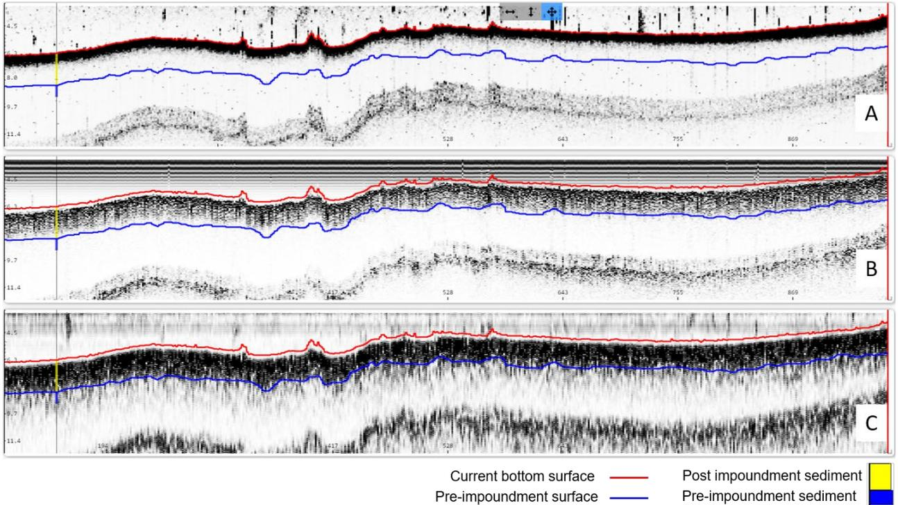
**Figure 8. Sediment core sample WX-7 compared with acoustic signal returns. A) 208 kHz frequency, B) 50 kHz frequency, and C) 12 kHz frequency.**
