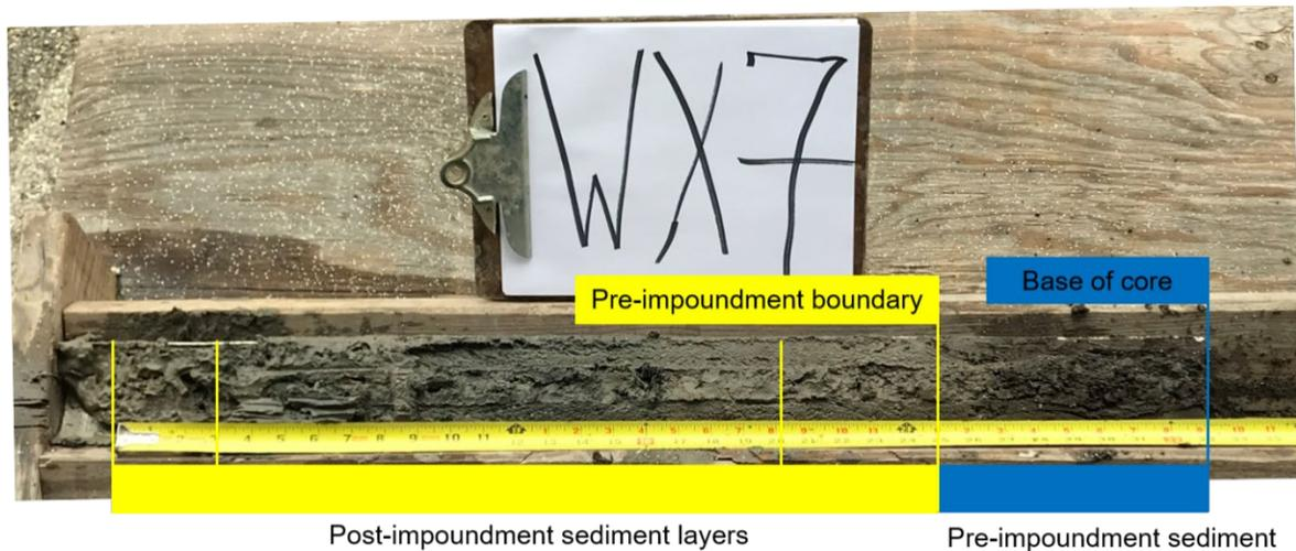
**Figure 7. Sediment cores WX-7. Post-impoundment sediment layers are identified by yellow boxes. Pre-impoundment sediment layers are identified by blue boxes.**
