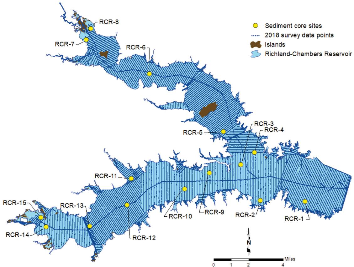
Figure 2. 2018 TWDB Richland-Chambers Reservoir survey data (blue dots) and sediment coring locations (yellow circles)
