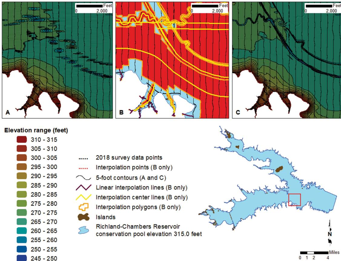
**Figure 3. Anisotropic spatial interpolation and linear interpolation of Richland-Chambers Reservoir sounding data; A) bathymetric contours without interpolated points, B) sounding points (black) and interpolated points (red), C) bathymetric contours with interpolated points.**
