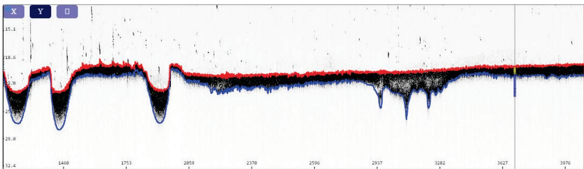
**Figure 9.** Cross-section of data collected during survey, displayed in Hydropick (208 kHz frequency), correlated with sediment core sample RCR-6 and showing the current surface in red and pre-impoundment surface in blue.
