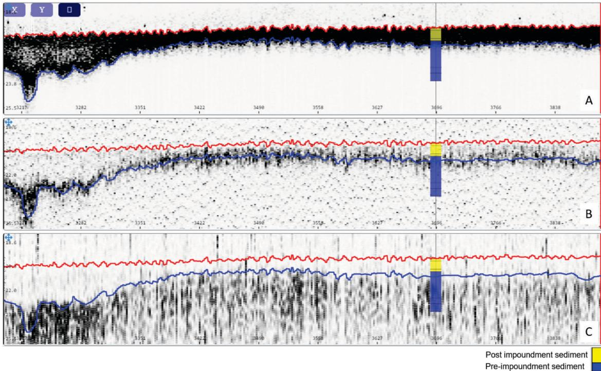
**Figure 8.** Comparison of sediment core RCR-6 with acoustic signal returns. A) 208 kHz frequency, B) 50 kHz frequency, and C) 12 kHz frequency. The current surface in red and pre-impoundment surface in blue.
