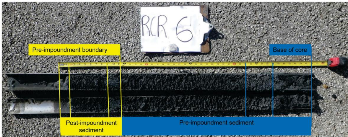
**Figure 7. Sediment core RCR-6 from Richland-Chambers Reservoir. Post-impoundment sediment layers occur in the top 11.0 inches of this sediment core (identified by the yellow box). Pre-impoundment sediment layers were identified and are defined by the blue box.**
