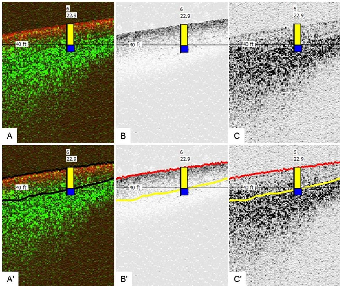
**Figure 8.** Comparison of sediment core PK-6 with acoustic signal returns A, A') combined acoustic signal returns, B, B') 208 kHz frequency, and C, C') 50 kHz frequency.
