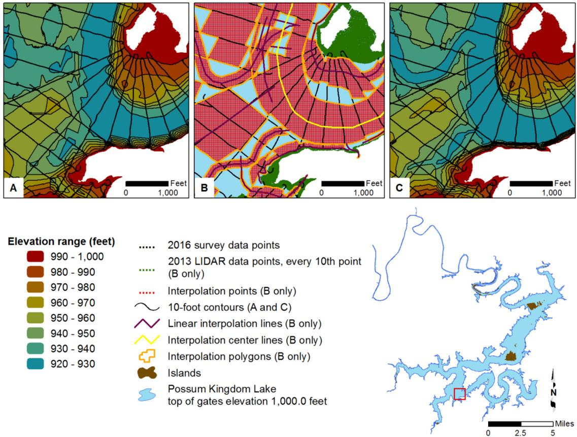
**Figure 3. Anisotropic spatial interpolation and linear interpolation of Possum Kingdom Lake sounding data; A) bathymetric contours without interpolated points, B) sounding points (black) and interpolated points (red), C) bathymetric contours with interpolated points.**
