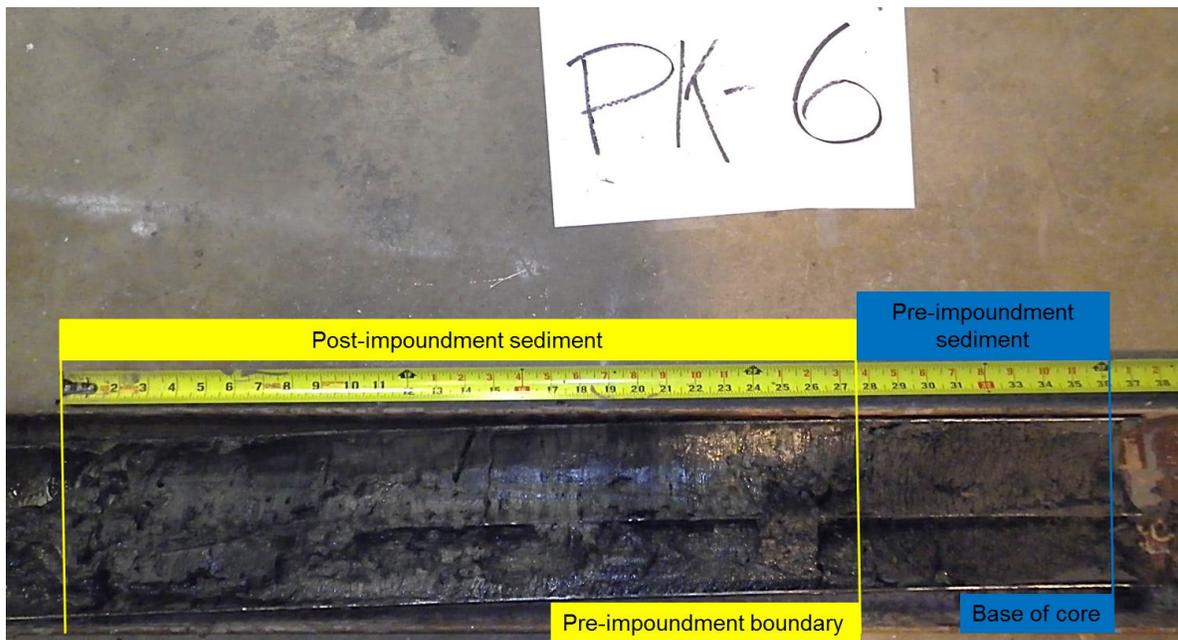
**Figure 7.** Sediment core PK-6 from Possum Kingdom Lake. Post-impoundment sediment layers occur in the top 27.5 inches of this sediment core (identified by the yellow box). Pre-impoundment sediment layers were identified and are defined by the blue box.
