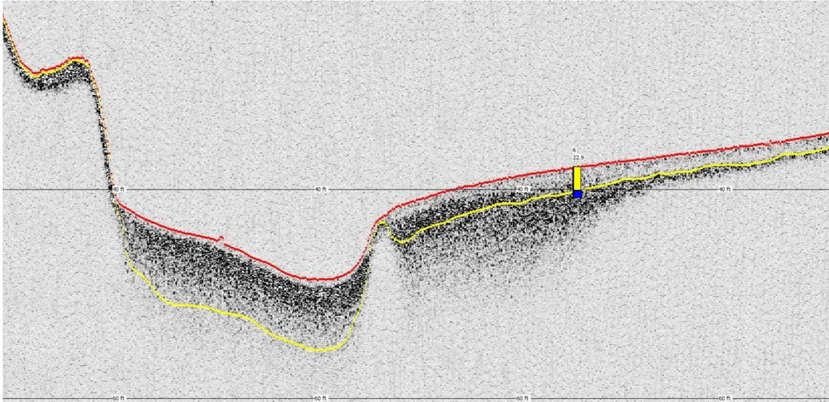
**Figure 9.** Cross-section of data collected during the 2016 survey, displayed in DepthPic© (50 KHz acoustic signal returns), correlated with sediment core sample PK-6 and showing the current surface as the top red line, and pre-impoundment surface as the bottom yellow line.
