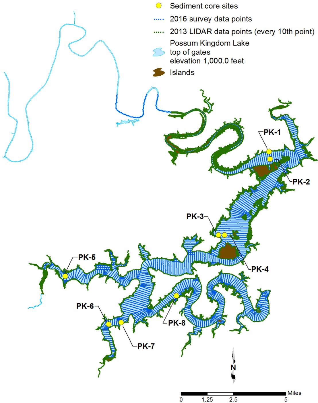
Figure 2. 2016 TWDB Possum Kingdom Lake survey data (*blue dots*) and sediment coring locations (*yellow circles*), and 2013 LIDAR data (*green dots*) between elevations 989.95 and 1,000.00 feet.
