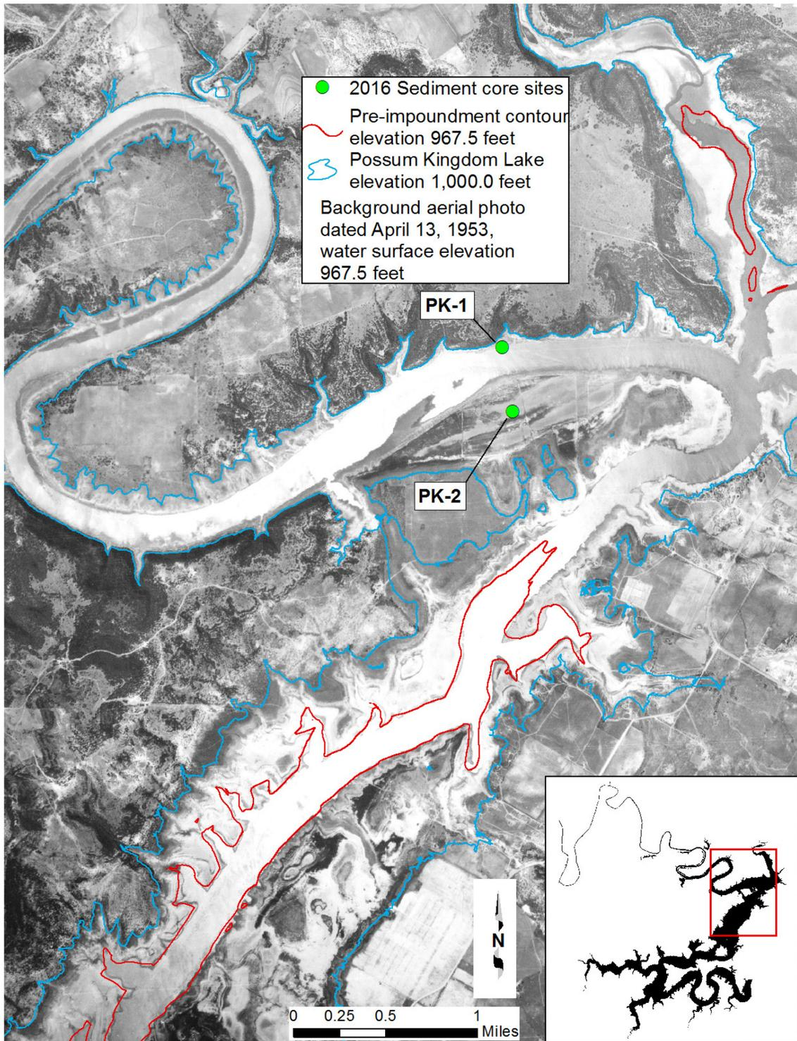
Figure 15. The TWDB surveyed pre-impoundment contour at elevation 967.5 feet (*red line*) overlain on an aerial photograph taken on April 13, 1953, while the daily average water surface elevation measured 967.5 feet. The current 1,000-foot contour is shown in blue. The TWDB sediment core samples PK-1 and PK-2 (*green dots*) were collected in this part of the lake.
