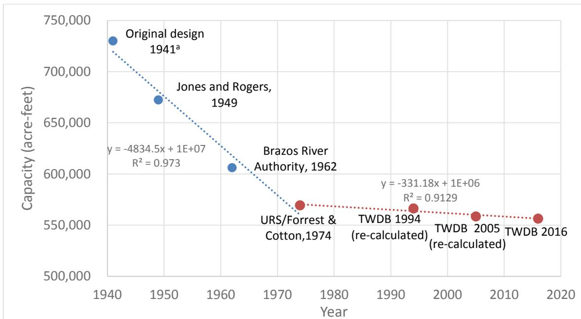
Figure 11. Plot of total capacity estimates at elevation 1,000.0 feet for Possum Kingdom Lake. Capacity estimates before 1974 shown as blue dots, and capacity estimates since 1974 shown as red dots. Blue and red trend lines illustrate a shift in rate of capacity changes before and after 1974.
