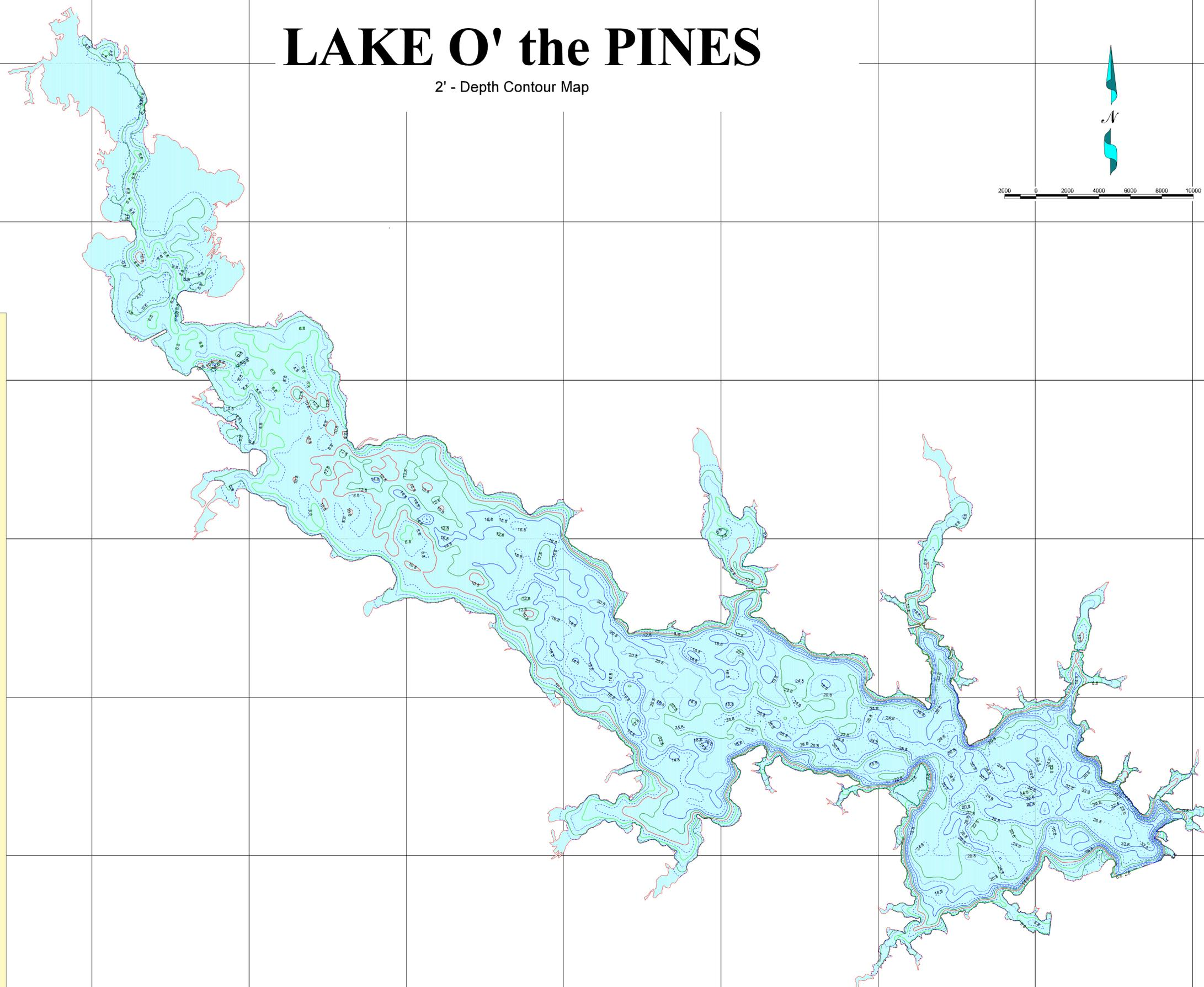
This map is the product of a survey conducted by the Texas Water Development Board's Hydrographic Survey Program to determine the capacity of Lake O' the Pines. The Texas Water Development Board makes no representations and assumes no liability if this information is used for other purposes such as boating maps.
