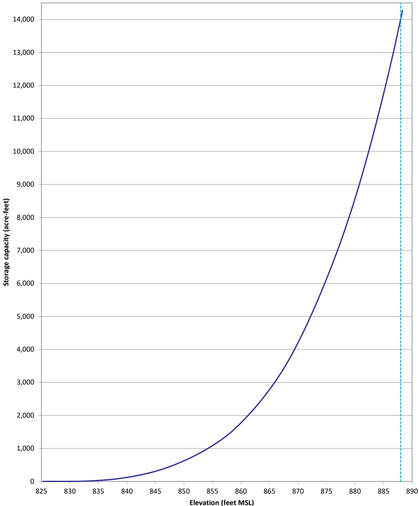
— Total bathymetric capacity 2021    - - - - Conservation pool elevation 888.0 feet MSL
