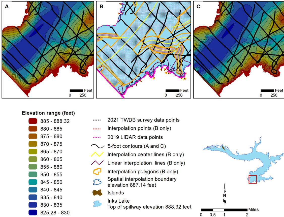
**Figure 3. Anisotropic spatial interpolation as applied to Inks Lake sounding data; A) bathymetric contours without interpolated points, B) sounding points (black) and interpolated points (red), C) bathymetric contours with interpolated points.**
