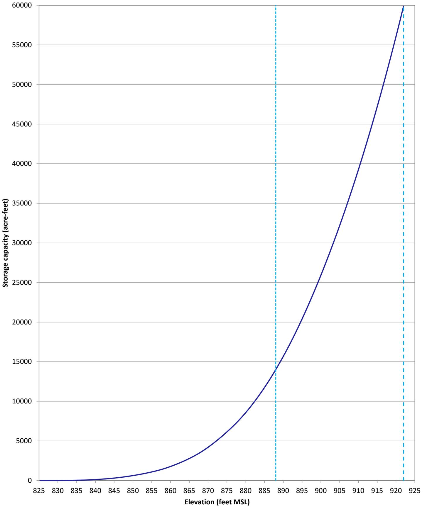
— Total bathymetric and topographic capacity 2021
