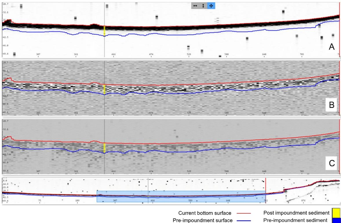
**Figure 8.** Comparison of sediment core IK-4 with acoustic signal returns. A) 208 kHz frequency, B) 50 kHz frequency, and C) 12 kHz frequency. The current surface in red and pre-impoundment surface in blue.
