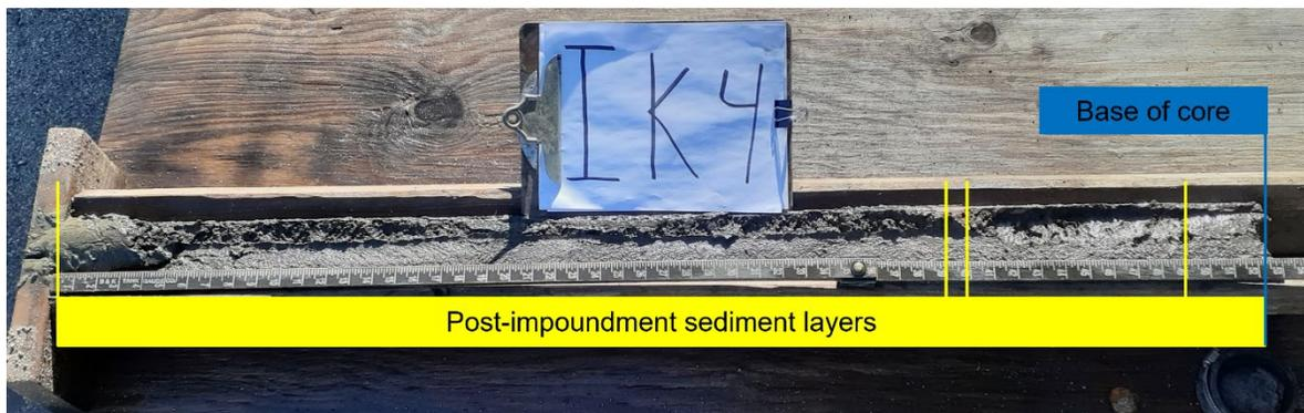
**Figure 7.** Sediment core IK-4 from Inks Lake. Post-impoundment sediment layers occur throughout the entire 53.0 inches of this sediment core (identified by the yellow box). The base of the core is denoted by the blue line.
