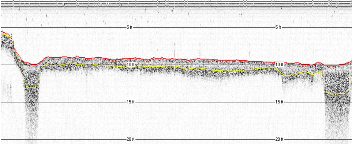
**Figure 6.** The 50 kHz signal profile in Reservoir B shows the approximate pre-impoundment boundary (yellow line) and ditches on each end of profile. The light gray and black-white speckled signal response was interpreted to be the sediment layer without corroboration with core samples. The lighter gray area is most probably a fine particle, low-density mud with high water content. See Figure 8 for location of profile.
