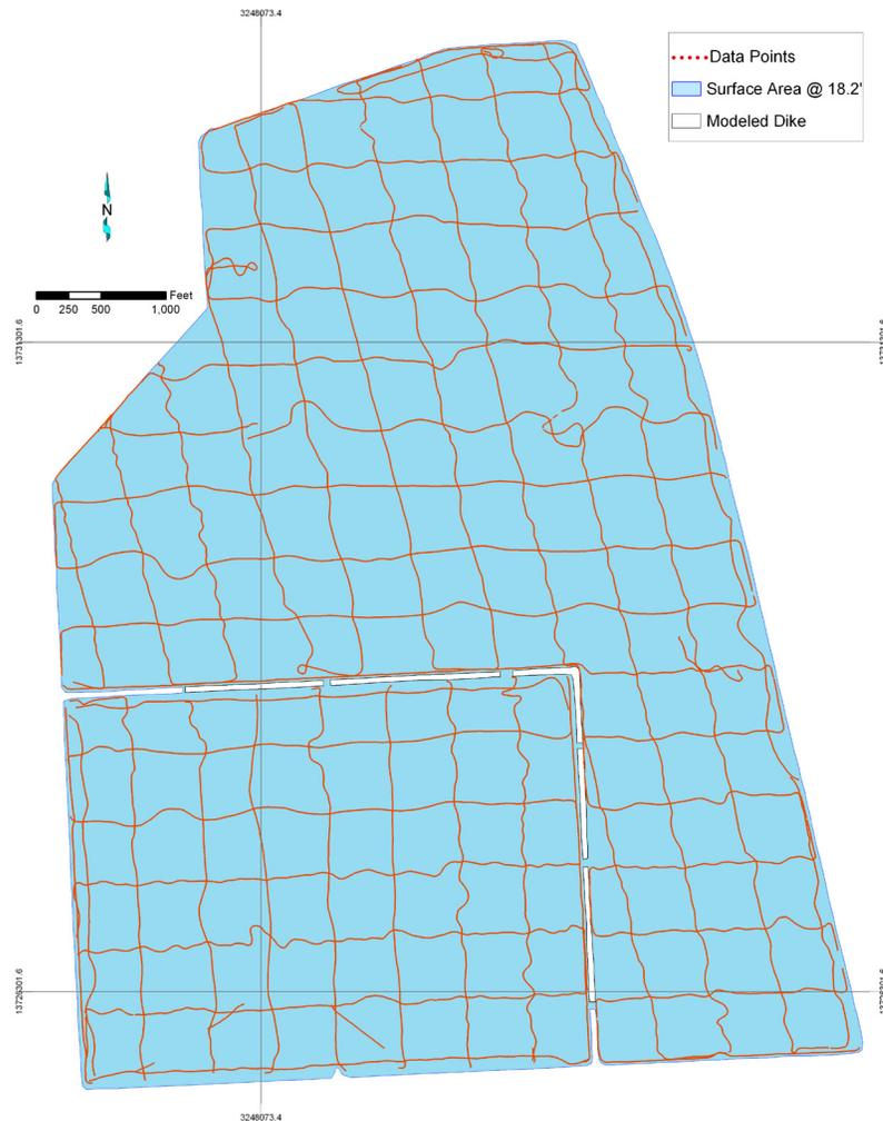
**Figure 3.** Location of data, collected in 500-foot grid pattern, in Gulf Coast Water Authority’s Reservoirs A and B. The six openings in the inner levee were incorporated to connect the reservoirs in the TIN model and are not drawn in their actual location in this figure.
