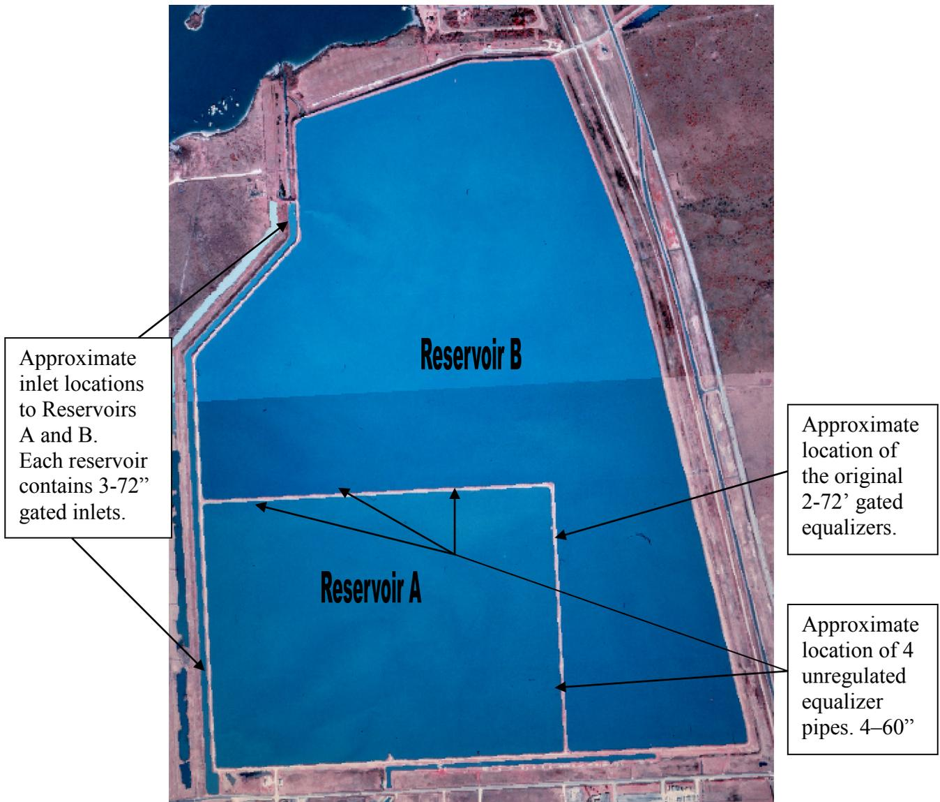
**Figure 2.** 1995 aerial photograph of Gulf Coast Water Authority’s Reservoirs A and B with a portion of Dickinson Bayou visible in the upper left hand corner. Additionally, the inner levee has equalizers below normal pool elevation joining the two reservoirs. See additional sketch in Appendix H.
