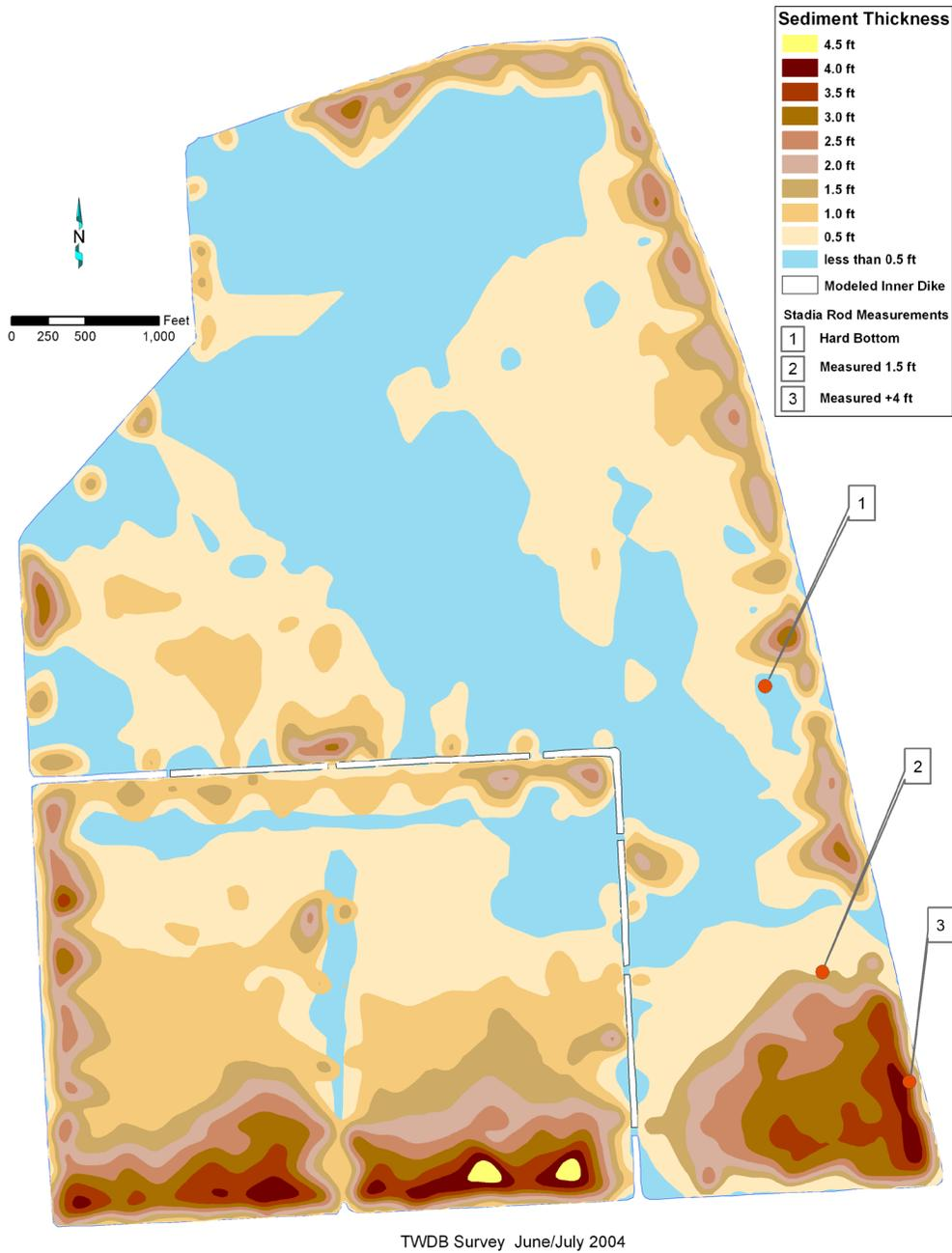
**Figure 4.** Estimated location and thickness of sediment found in Reservoirs A and B.
