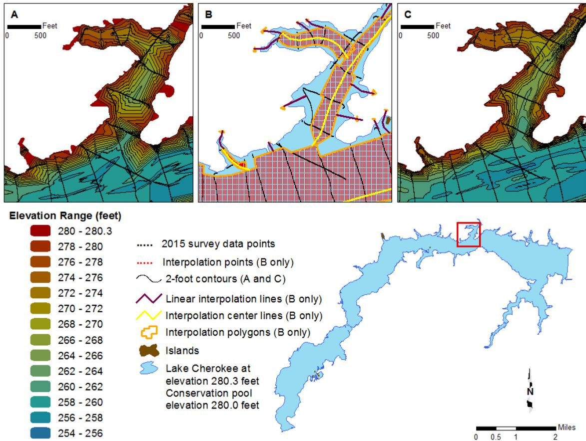
**Figure 3. Anisotropic spatial interpolation and linear interpolation of Lake Cherokee sounding data - A) bathymetric contours without interpolated points, B) sounding points (black) and interpolated points (red), C) bathymetric contours with the interpolated points**
