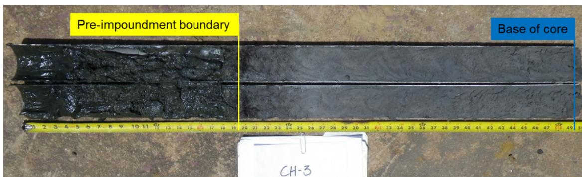
**Figure 7. Sediment core sample CH-3 from Lake Cherokee**
