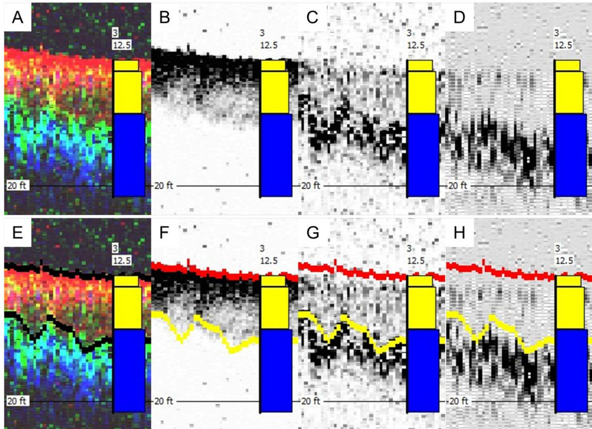
**Figure 8. Comparison of sediment core sample CH-3 with acoustic signal returns: A,E) combined acoustic signal returns, B,F) 208 kHz frequency, C,G) 50 kHz frequency, D,H) 24 kHz frequency**
