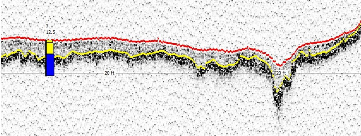
**Figure 9. Cross-section of data collected during survey, displayed in DepthPic© (50 kHz frequency), correlated with sediment core sample CH-3 and showing the current surface in red and pre-impoundment surface in yellow**
