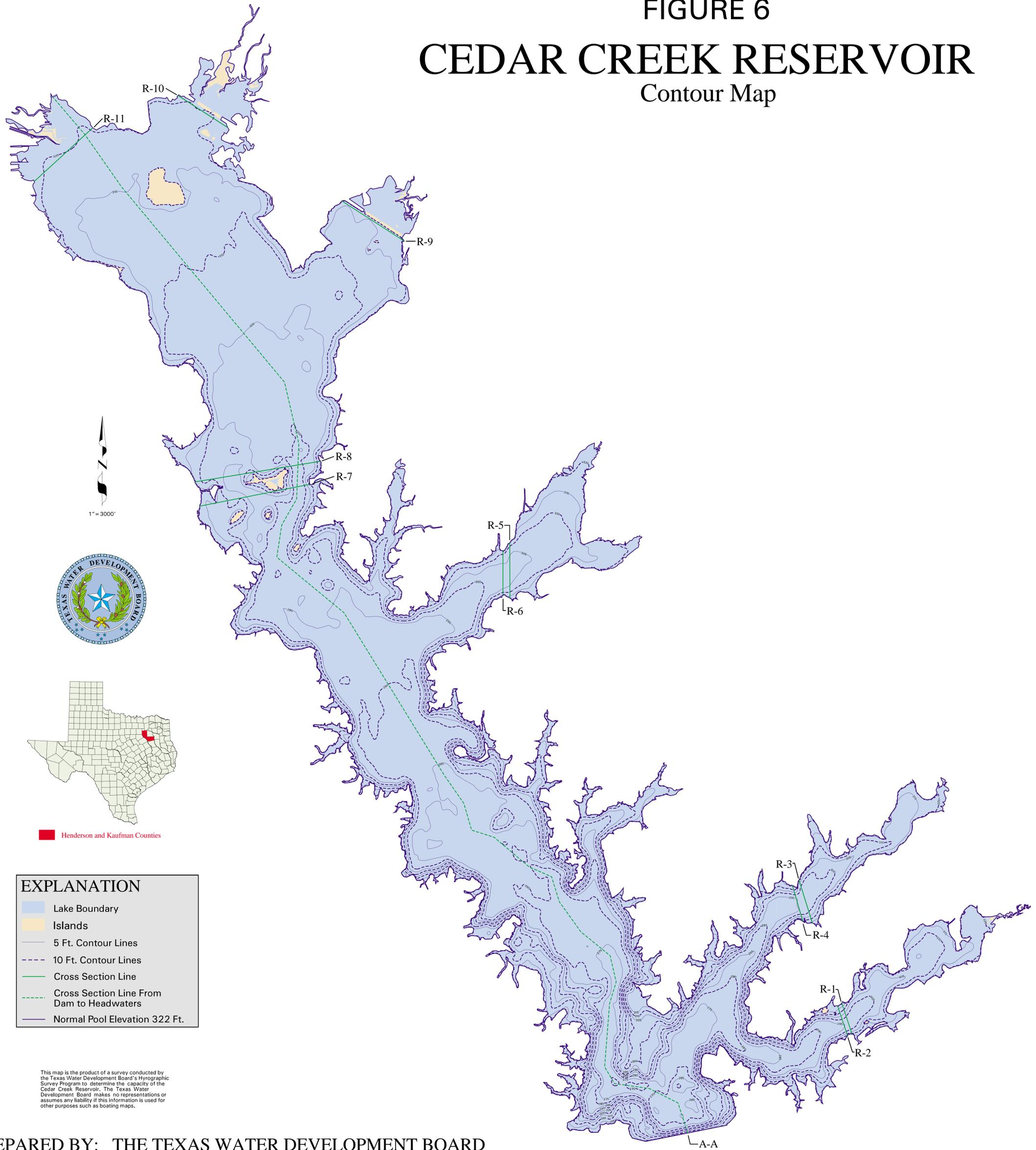
This map is the product of a survey conducted by the Texas Water Development Board's Hydrographic Survey Program to determine the capacity of the Cedar Creek Reservoir. The Texas Water Development Board makes no representations or assumes any liability if this information is used for other purposes such as boating maps.
