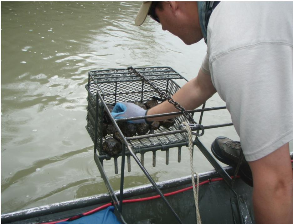
**Figure 21.** Small dredge used for mussel sampling in deep areas.
