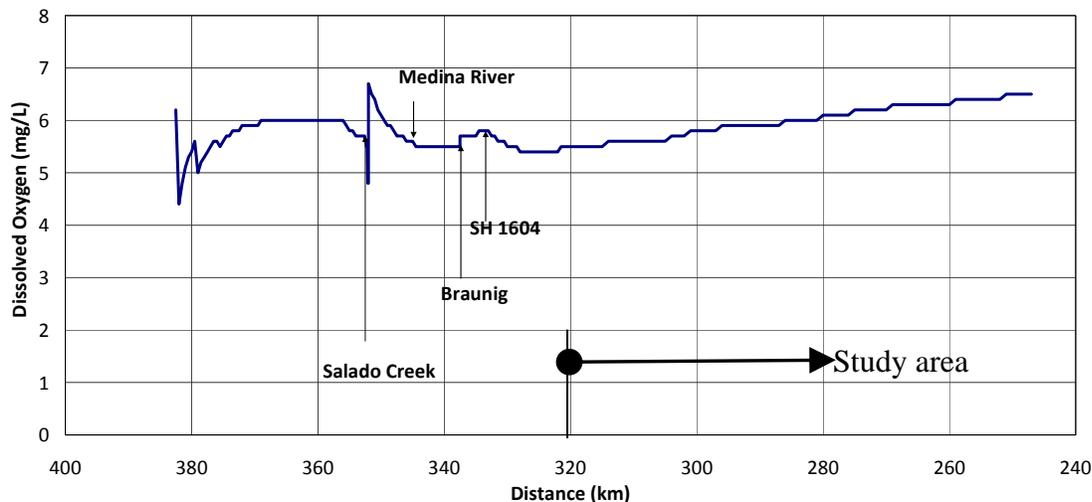
**Figure 34.** Dissolved Oxygen longitudinal profile - LSAR upper segment with 100 cfs flow after diversion at Braunig, with zero headwater flows and water temperature of 33.2 °C.
