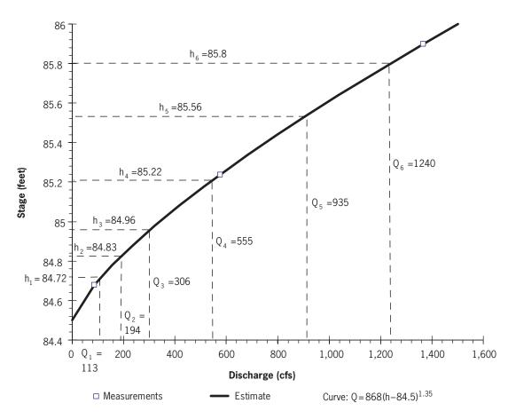
Figure 6-3. Stage-discharge curve developed for hydraulic model input. cfs=cubic feet per second, 35.3 cubic feet per second is equal to 1 cubic meter per second
