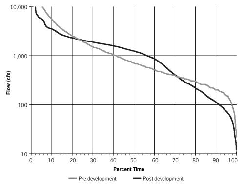
Figure 6-1. Flow duration curve calculated from daily data for pre-development and post-development conditions.
