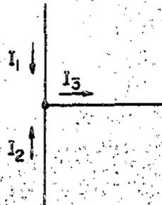
The electric system shown on the right illustrates Kirchoff's Current Law, which states that the sum of currents flowing into a junction equals the sum of currents flowing out of the junction.
