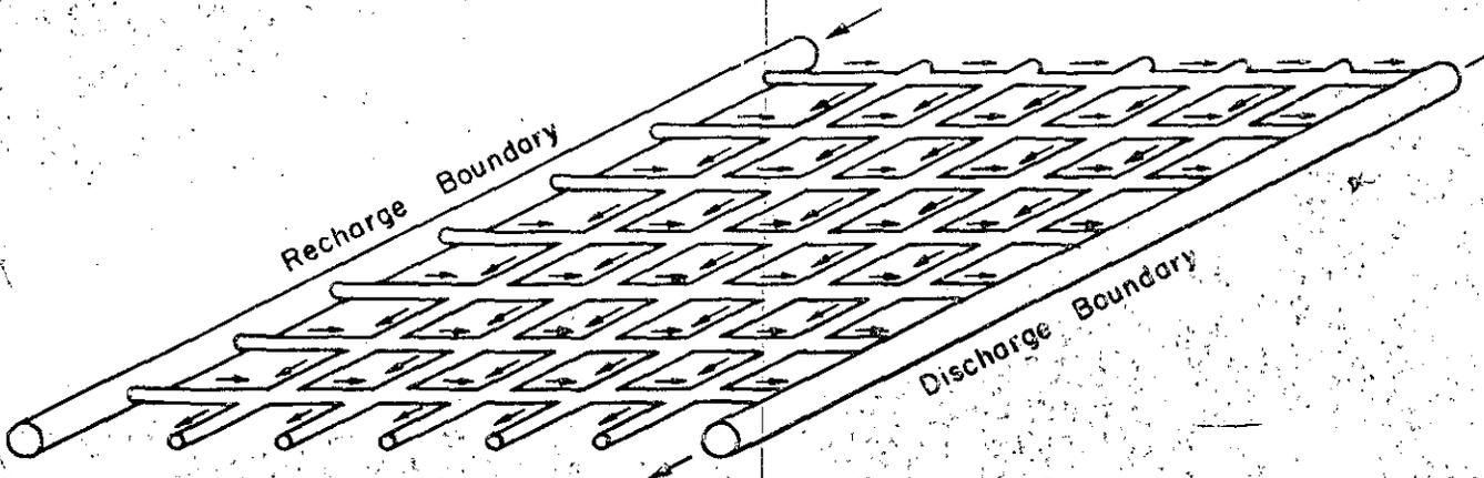
The pipe-network system of fluid flow can be modeled with a resistor-network system of electric flow.
