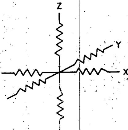
Electric-analog models are advantageous in the study of flow problems involving non-uniform permeability and irregularly-shaped boundaries.
