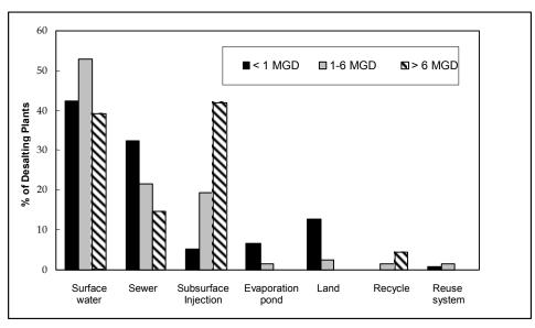
Figure 7 Percentage of desalting plants >0.025 MGD by disposal method and capacity (Mickley, 2004a)
