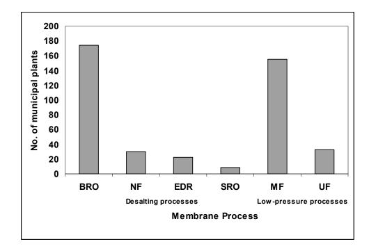
Figure 2-Number of municipal membrane plants of different types >0.025 MGD built prior to 2003 (Mickley, 2004a)
