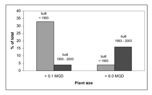
Figure 5 Changes in municipal membrane plant size before and after 1993 (Mickley, 2004a)
