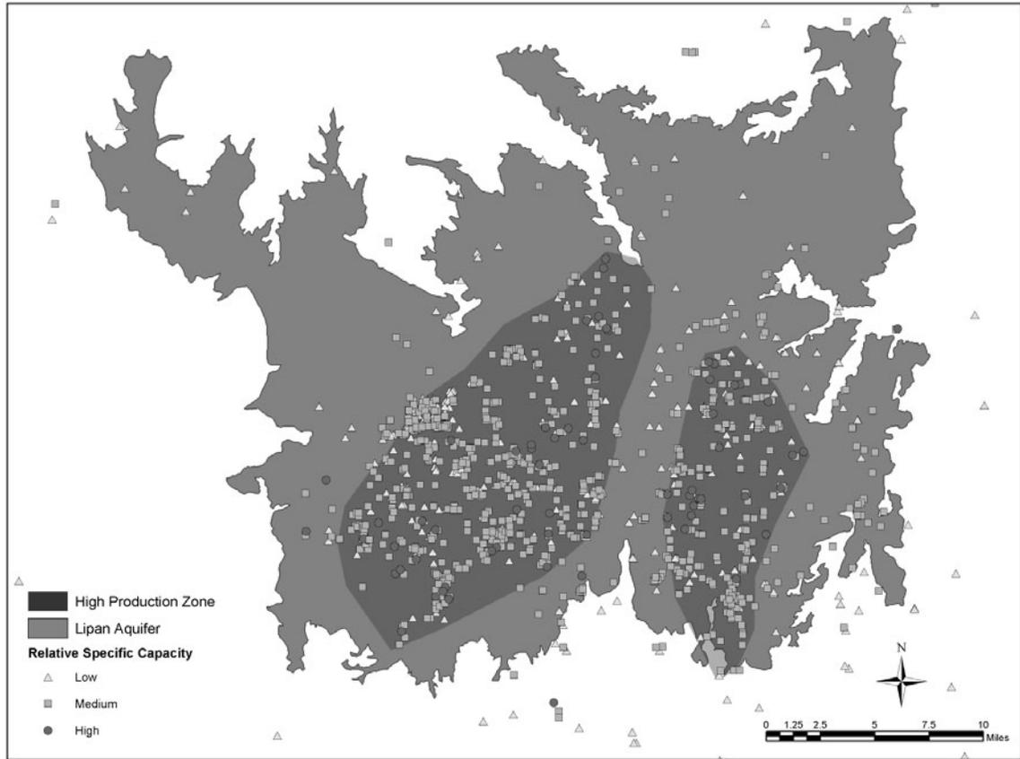
Figure 8-7: Distribution of specific-capacity values calculated from production capacity (ft<sup>2</sup>/day) and the log distribution of these values in the Lipan aquifer.
