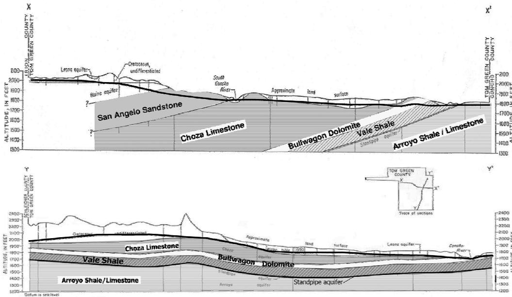
Figure 8-6: Geologic cross-sections of the Lipan Aquifer (after Lee, 1986).
