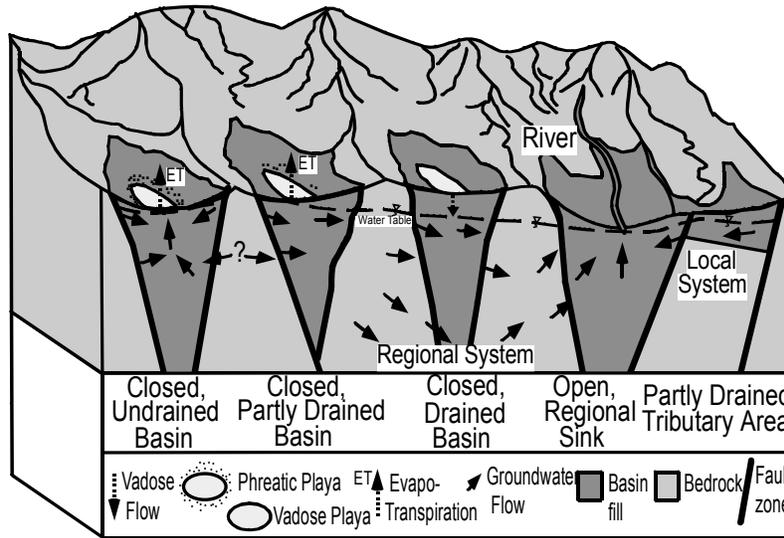
Figure 7-4: Schematic diagram showing hydrogeologic framework and groundwater-flow system in interconnected group of *closed* and *open, undrained, partly drained, and drained* intermontane basins (modified from Eakin and others, 1976, and Hibbs and others, 1998).
