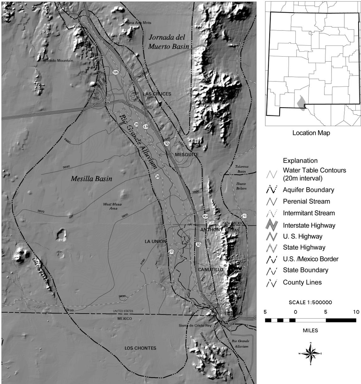
Figure 7-2: Shaded-relief index map of the Mesilla Basin area of southern New Mexico and adjacent parts of Texas and Chihuahua showing extent of modeled basin-fill (Santa Fe Gp) and Mesilla Valley aquifer systems. General water-table configuration and groundwater-flow direction in upper aquifer units are also illustrated (adapted from Hibbs and others [1997], with shaded relief from latest available U.S. Geological Survey DEM database).
