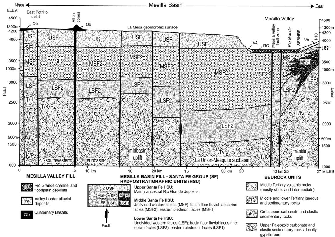
Figure 7-7: Schematic hydrogeologic cross section of the south-central Mesilla Basin near the 32<sup>nd</sup> Parallel in Doña Ana County, New Mexico, and El Paso County, Texas; with a vertical exaggeration of about 10× (modified from Hawley and Lozinsky, 1992).
