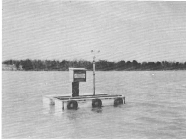
A. Standard Raft with Thermograph and Totalizing Anemometer
