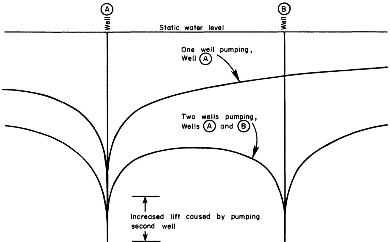
**Figure 12—Idealized Cross Section Showing Drawdown Interference Between Two Pumping Wells**
