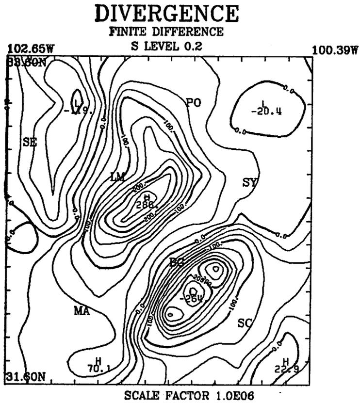
Fig. 4. Differential evaluation of divergence, by centered differences, for the HIPLEX region. Isopleth interval is  $25.0 \times 10^{-6} \text{ s}^{-1}$ .
