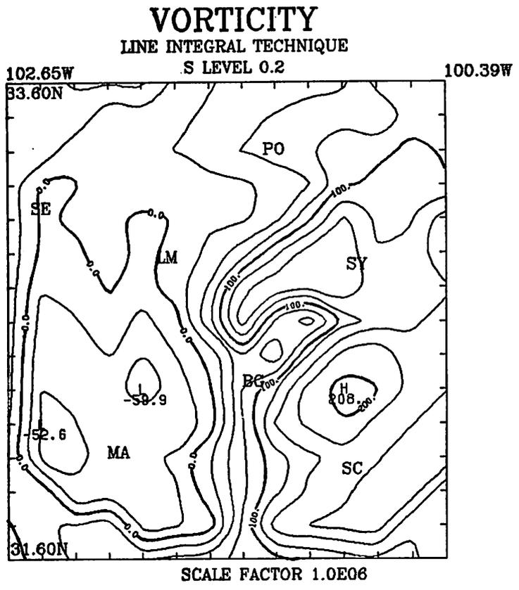
Fig. 10. LIT evaluation of vorticity for the HIPLEX region. Isopleth interval is  $25.0 \times 10^{-6} \text{ s}^{-1}$ .
