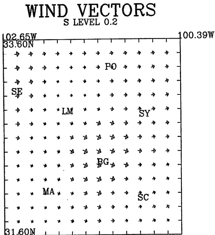
Fig. 3. Wind direction analysis of the original gridded wind field over the HIPLEX region. Size of arrowhead indicates relative magnitude of wind speed.
