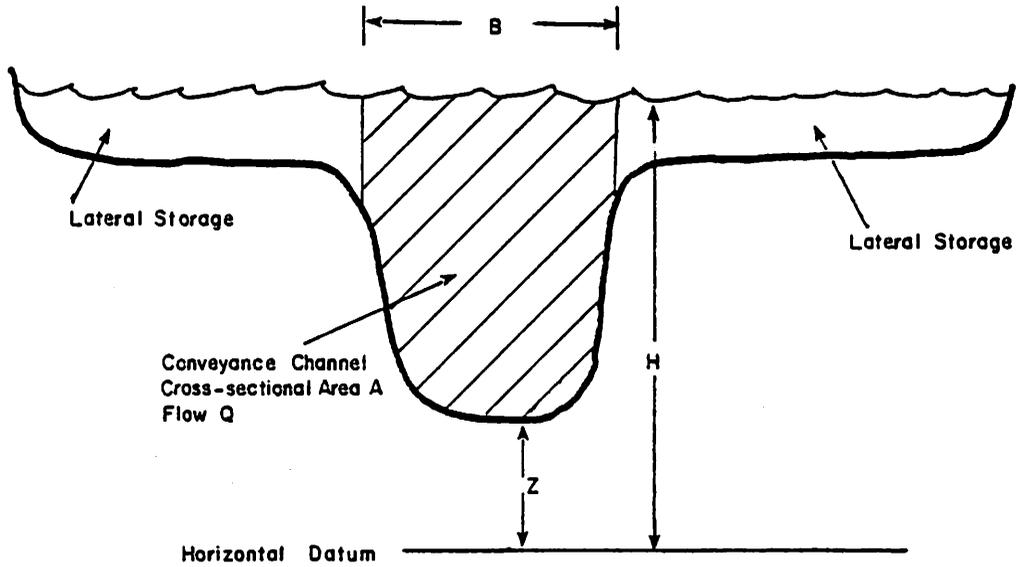
Figure II-2. Definition of Variables in Cross Section
