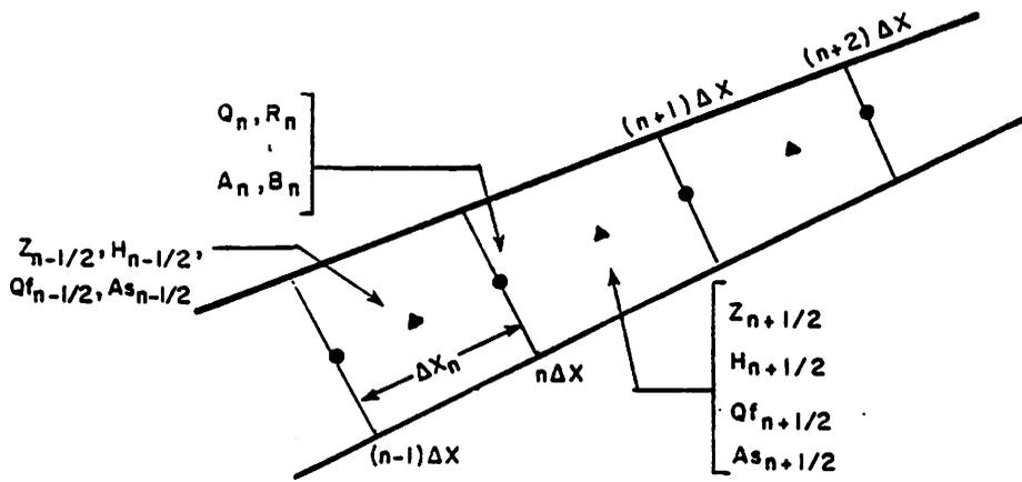
Figure II-3. Variable Definition in Finite-Difference Segmentation
