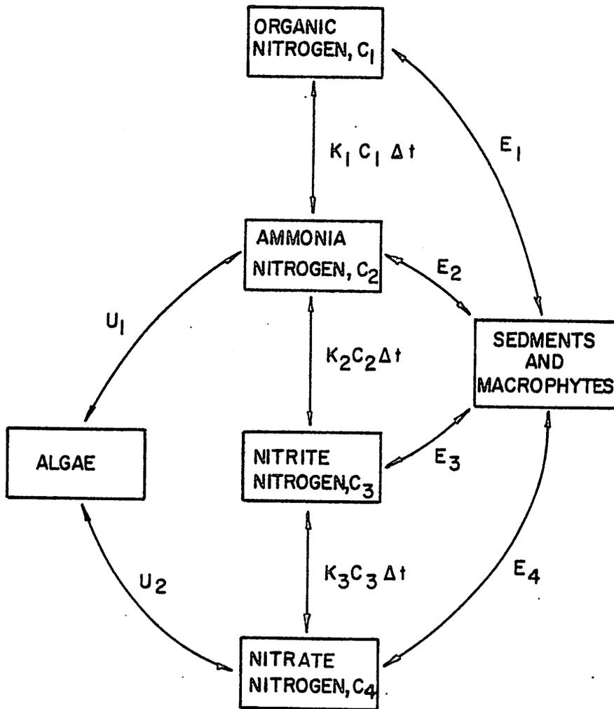
Figure III-1 NITROGEN CYCLE AS FORMULATED FOR MASS TRANSFER MODEL (Source: Hauck, 1977)
