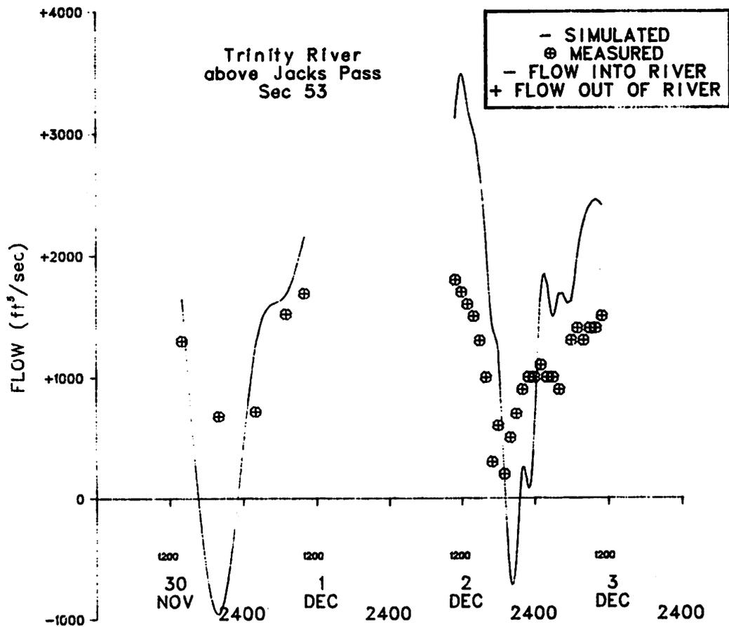
Figure II-35. Comparison of Measured and Simulated Flows.
