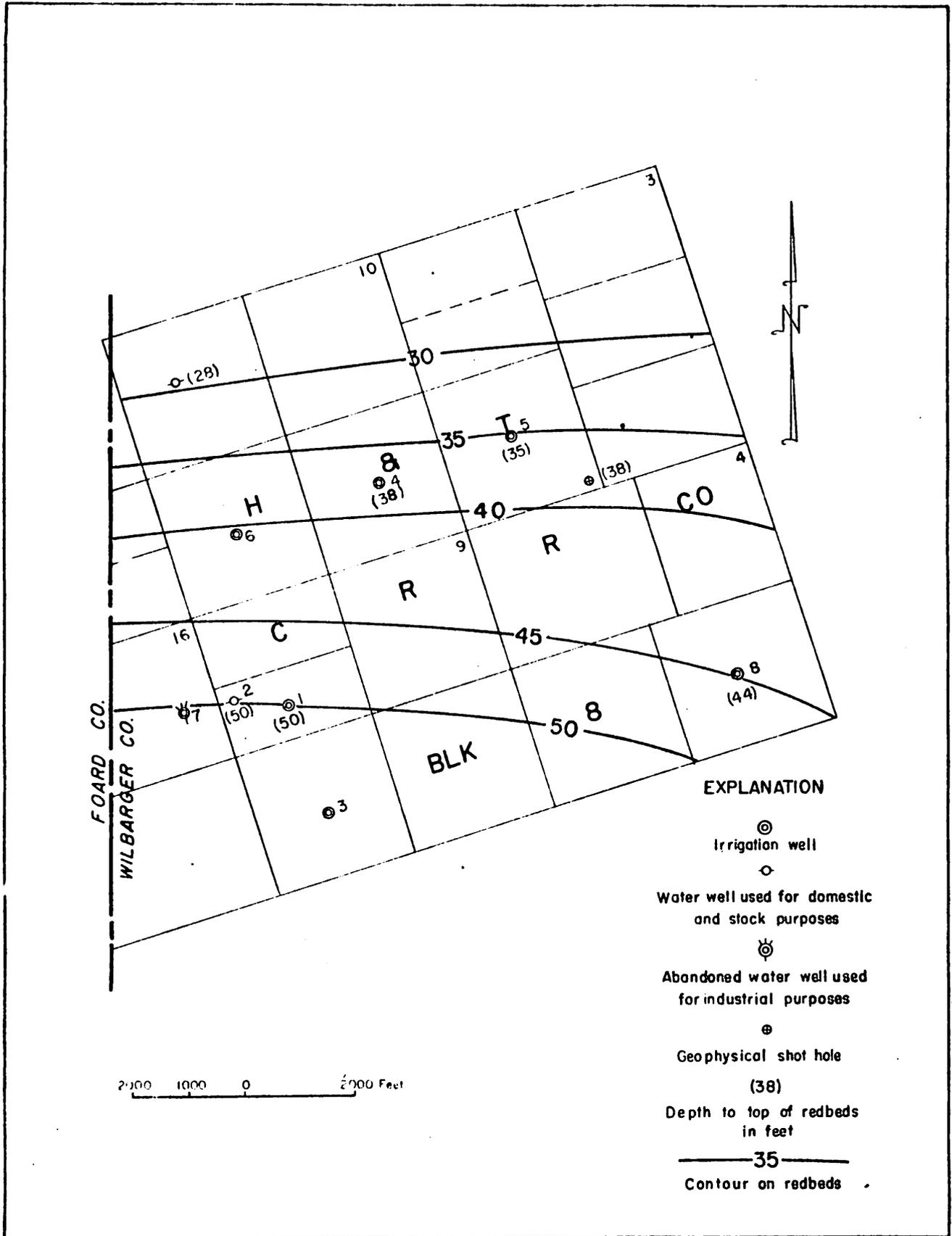
FIGURE 2.- Configuration of the Redbed Surface in area of Investigation, Wilbarger County, Texas
