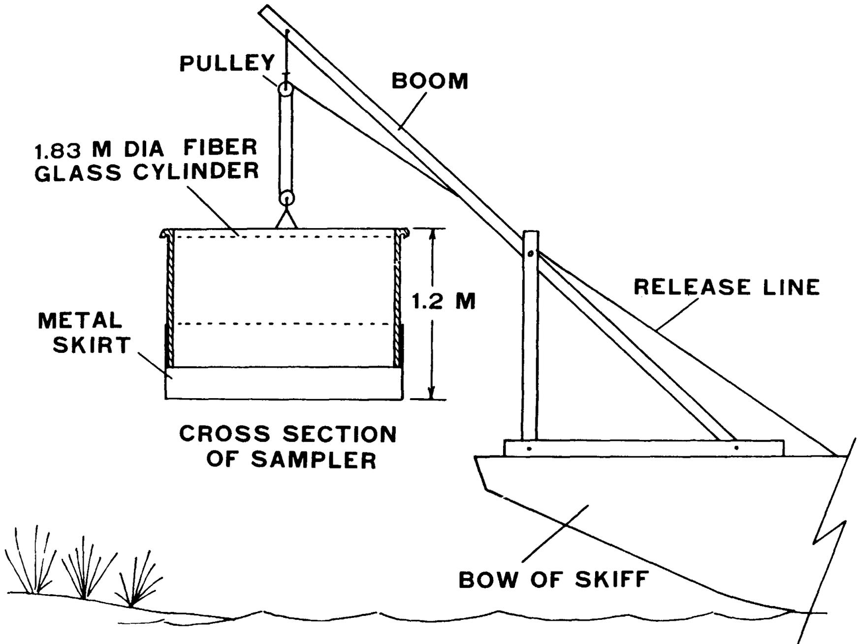
FIGURE 2. Drawing of the drop trap sampler.
