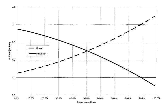
Figure 6 - Runoff/Infiltration for Various Levels of Impervious Cover for the 2 Year, 3 Hour Rainfall<sup>89</sup>
