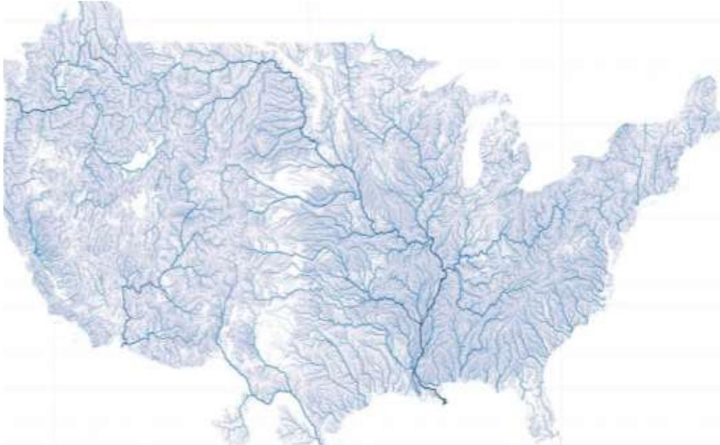
**Figure 5-8** NWM prediction of streamflow along streams in the NHD-plus database.
