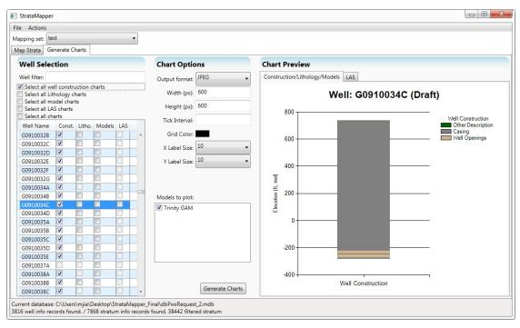
Figure 4-10 Export well construction charts in batch mode.
