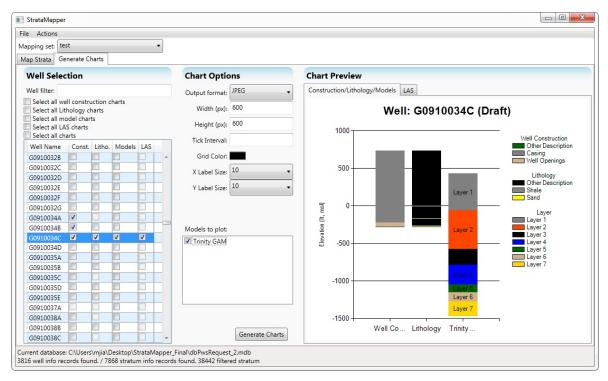
Figure 4-8 Preview of construction, lithology and model of well "G0910034C". Note that the "Sand" and "Shale" strata groups we specified before are used in the chart.
