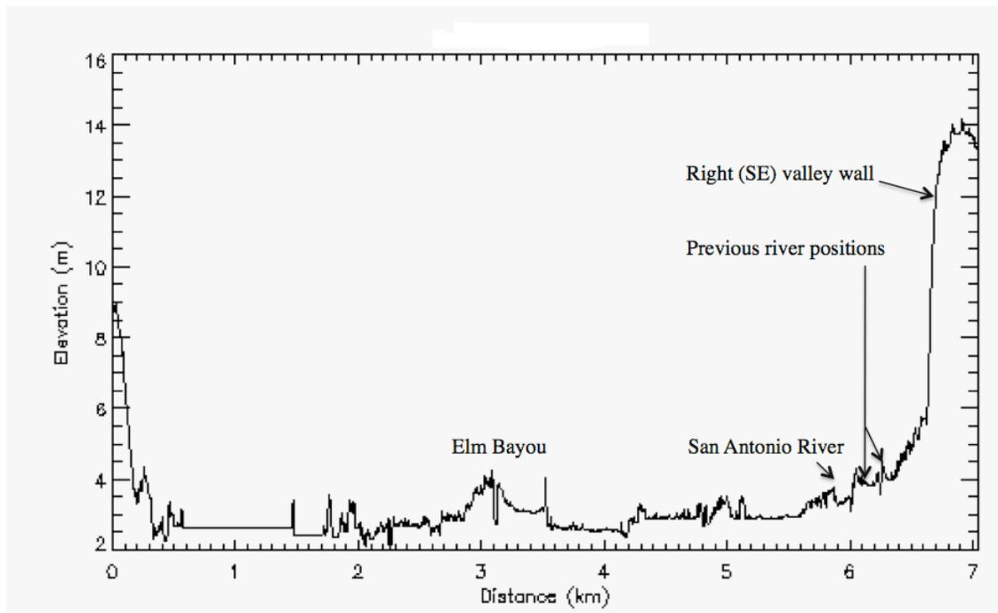
Figure 34. Topographic cross-section across the delta downstream of the San Antonio-Elm Bayou split. Note the former channel positions, and the backswamp and flood basin areas below the elevation of the channel beds.
