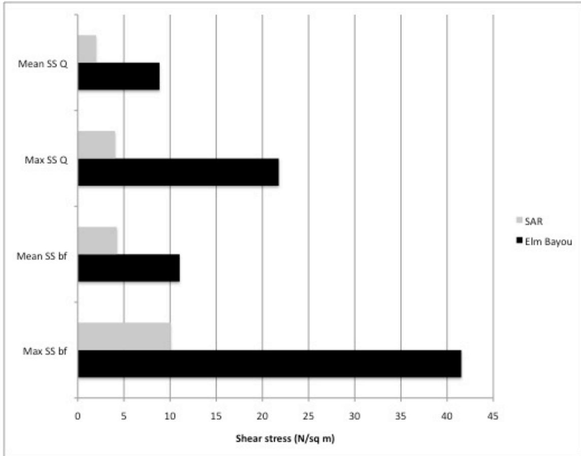
Figure 35. Differences in mean boundary and maximum bed shear stress (SS) for bankfull or banktop conditions (bf) and flow conditions at the time of measurement (Q) for Elm Bayou and the San Antonio River (SAR) downstream of the flow split.
