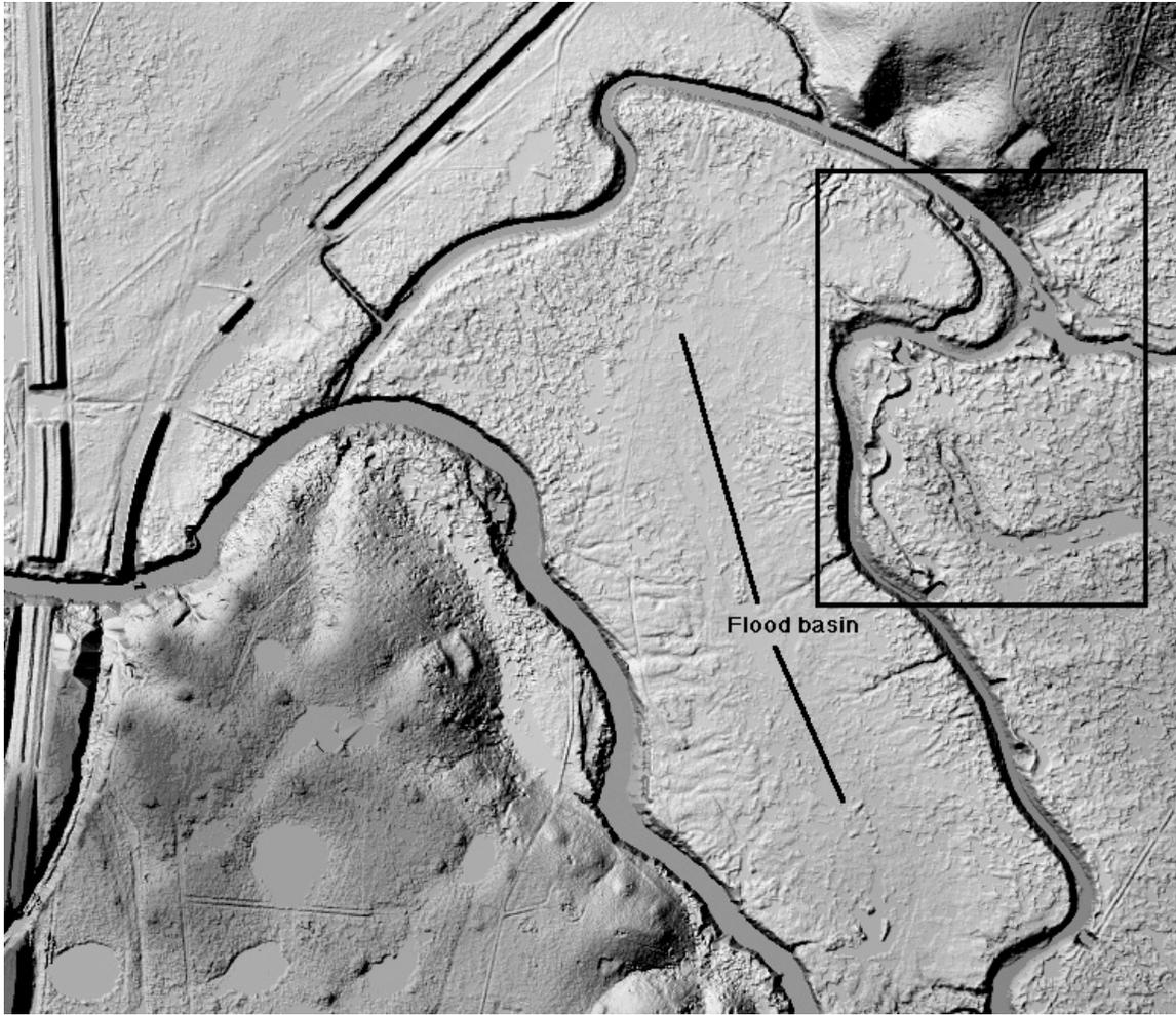
Figure 33. Shaded relief map of the upper San Antonio River Delta, showing a low-lying flood basin between the San Antonio and Old River alluvial ridges, and an avulsion node (box) at the Old River-Cushman Bayou junction. Note the paleochannels in the lower right area of the box, and paralleling the main channels.
