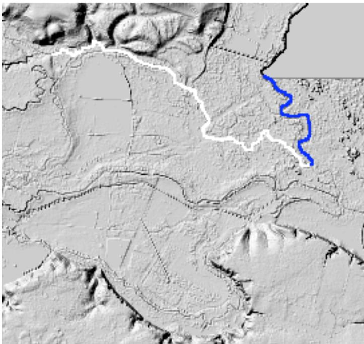
Figure 16. Path of Kuy Creek (white) to the Guadalupe River (blue) in its lower reaches. The channel in a portion of this reach has been obscured by modifications described in the text; the path is based on a flow routing algorithm for those sections.
