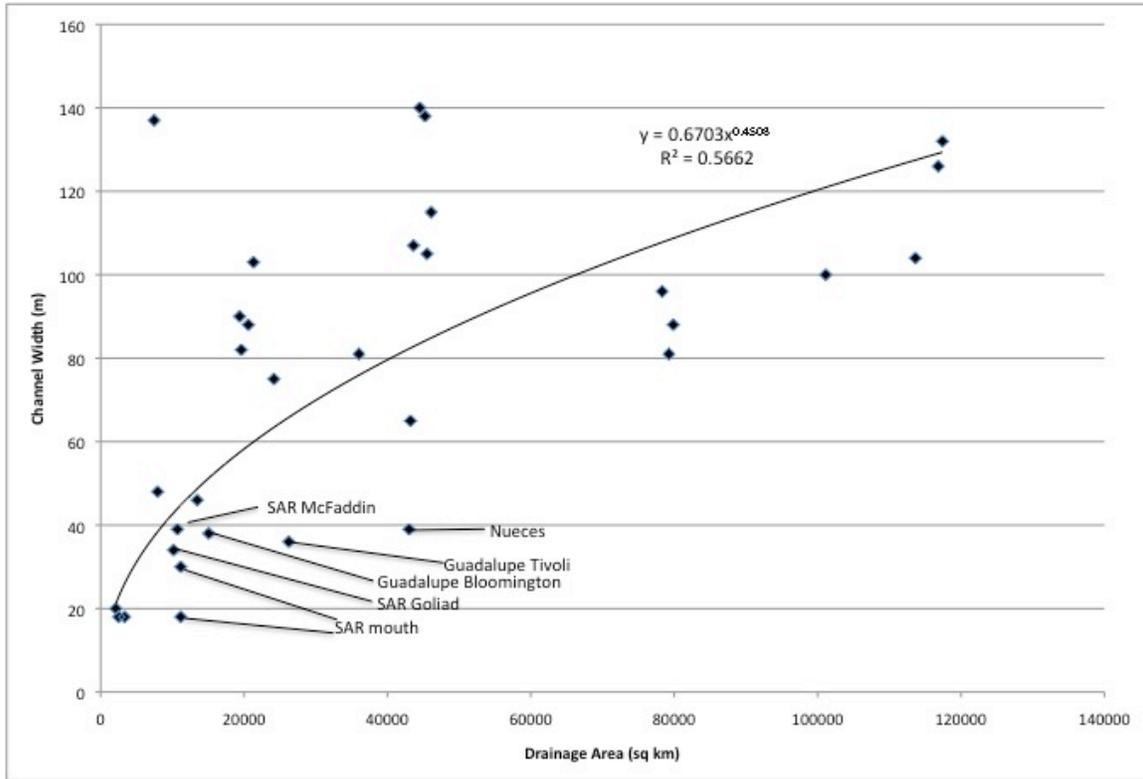
Figure 31. Relationship between channel width and drainage area for gaging stations on the lower reaches of 11 Texas rivers (see text). SAR = San Antonio River. The SAR mouth data points include Elm Bayou and the SAR. The best-fit regression is also shown.
