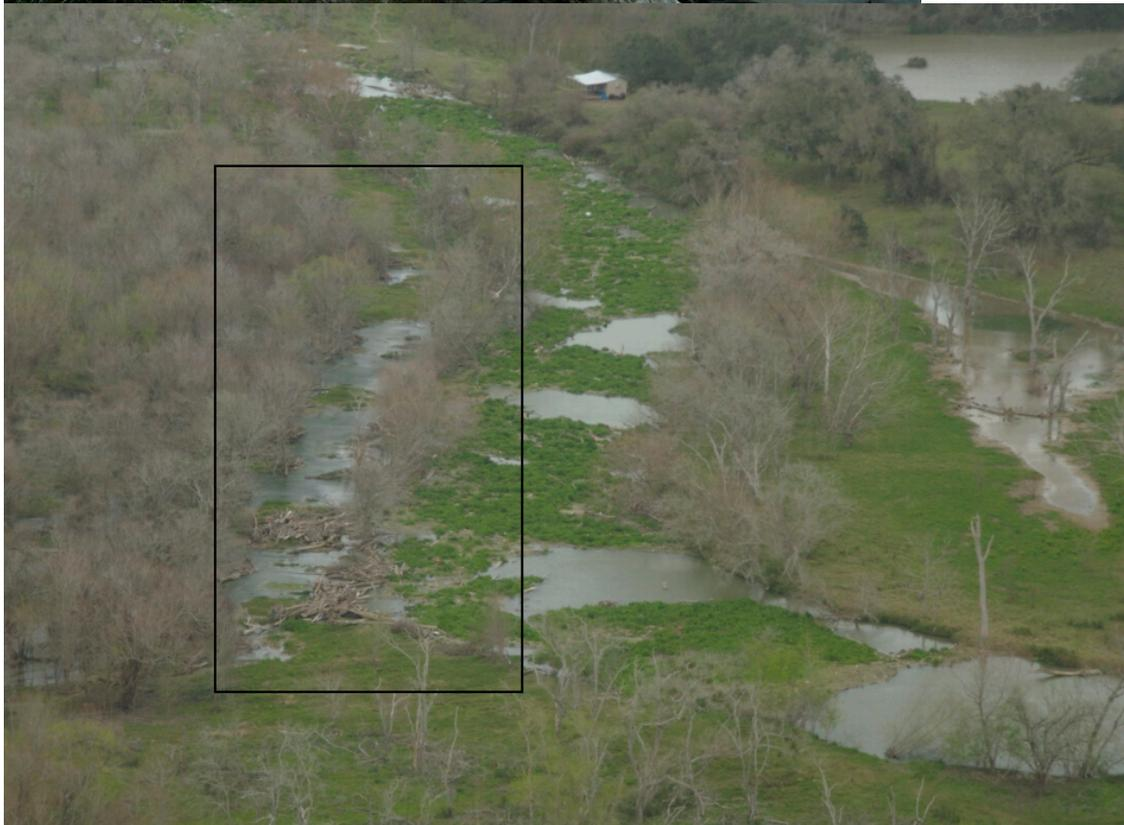
Figure 22. Bank erosion caused by flow deflection at the margin of the logjam (top). Channel widening by lateral flow displacement over a forested levee (bottom). The boxed area shows the forested levee top and former channel bank, with the new channel area established outside (left). The main, wood-jammed channel is to the right of the box. Note the new wood accumulations in the displaced channel. (Flow is toward the top of the photograph; photo by Walter Womack, February 2008).
