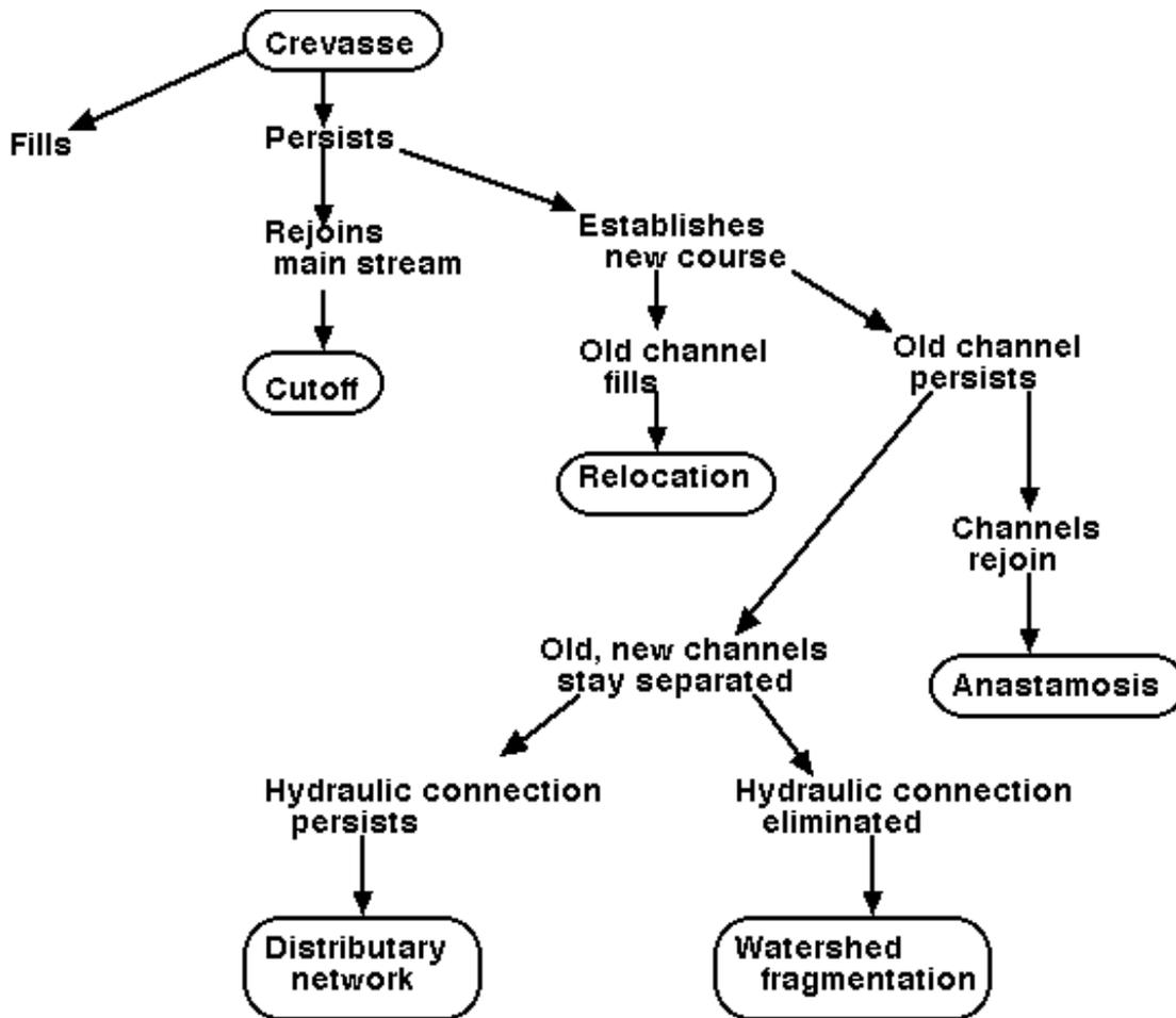
Figure 1. Possible outcomes of a crevasse that cuts a channel (as opposed to a splay or fan deposit).
